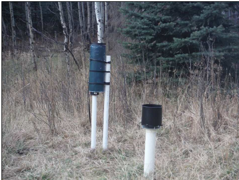
Figure 4: Initial site install of tipping bucket 1 and the totalizing gauge at BT, fall 2013; site was reconfigured and fencing was added approximately one year later.
