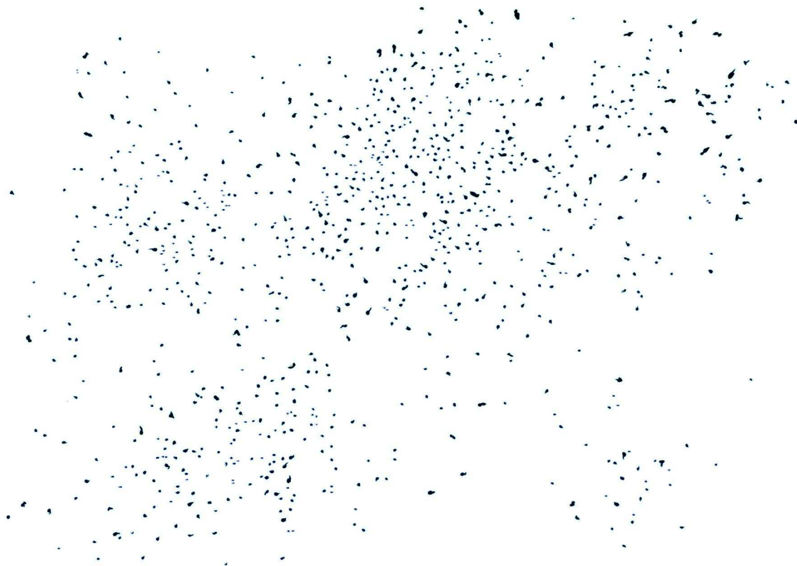
Figure 2.9. The result of analysis by ImageJ, Figure 2.8 was converted to black and white and each particle was counted. Image shows 941 bulbils, the blue color in the image are overlaid numbers identifying each individual bulbil; the actual size of this image is 4613 x 3255 pixels.
