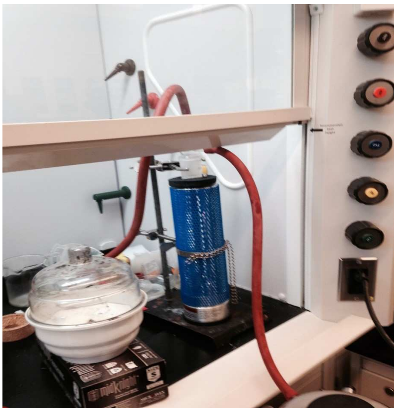
Figure 2.1.3: Glutaraldehyde vapor treatment setup.
