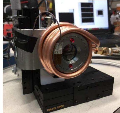
Figure 3-20: IR pyrometer with cooling jacket and surface thermocouple
