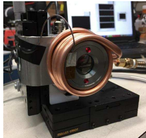
Figure B-18: IR pyrometer with cooling jacket and surface thermocouple.
