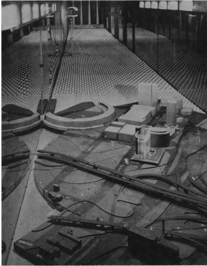
Figure 5a. Completed Model in the Wind Tunnel
