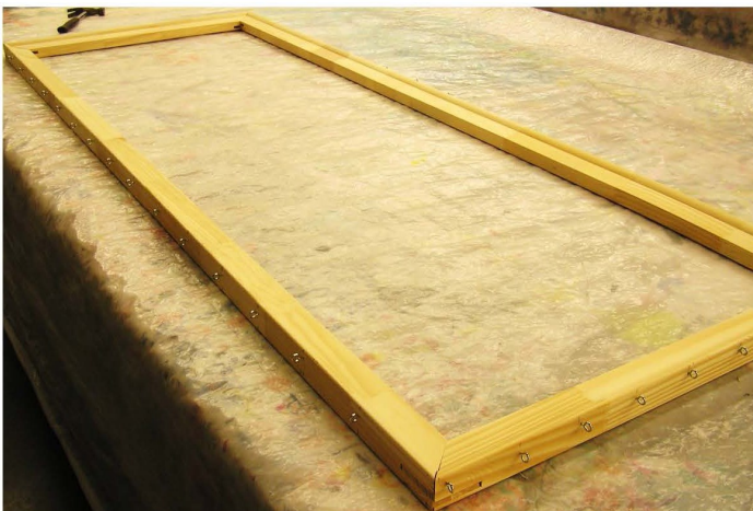
Assembling the frame and stringing the elastic cording through the eyelets
