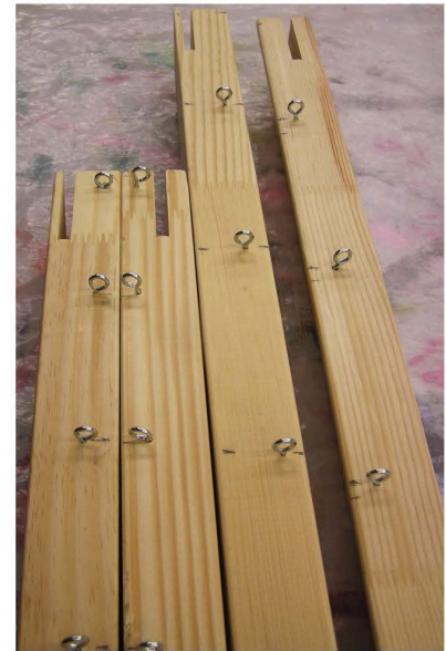
Screwing in the eyelets 8-10" apart.
