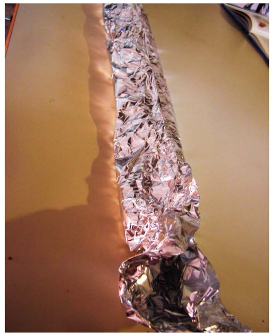
The rolled up silk on top of aluminum foil, and then sealed tightly at both ends.
