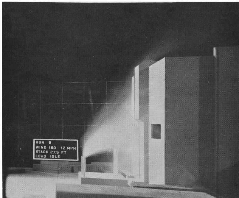
FIGURE 18. FLOW VISUALIZATION OF THE PLUMES FROM 27.5 FT STACKS (RUN 8, WD = 180°, U_R = 12 MPH, IDLE LOAD)
