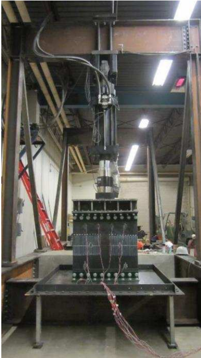
Figure 19. A physical front view of the test setup including the actuator, self-reacting frame, the base plate of the acrylic tank and the tested specimen
