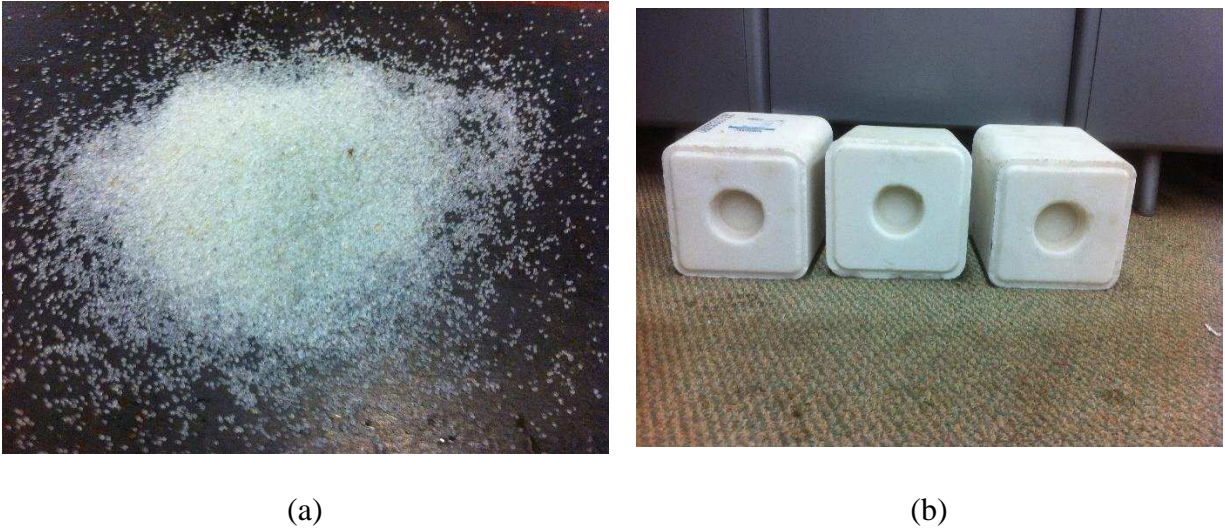
Figure 22. (a) 0.45-0.55 mm sand used (b) 23 kg (50 lbs) NaCl salt blocks
