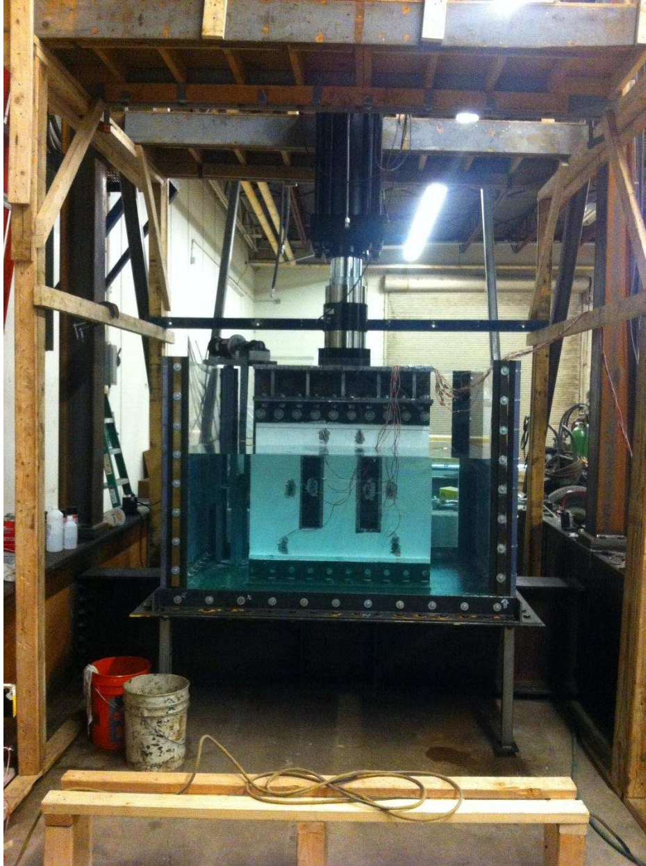
Figure 20. A physical front view of the test setup including the actuator, self-reacting frame, base plate with acrylic tank with water and tested specimen
