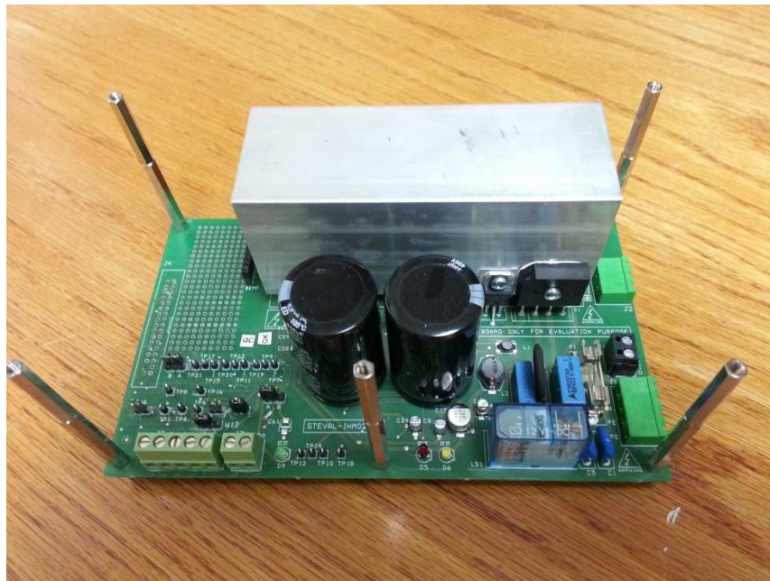
Figure 9: ST STEVAL-IHM025V1 1kW 3-phase motor control demonstration board
