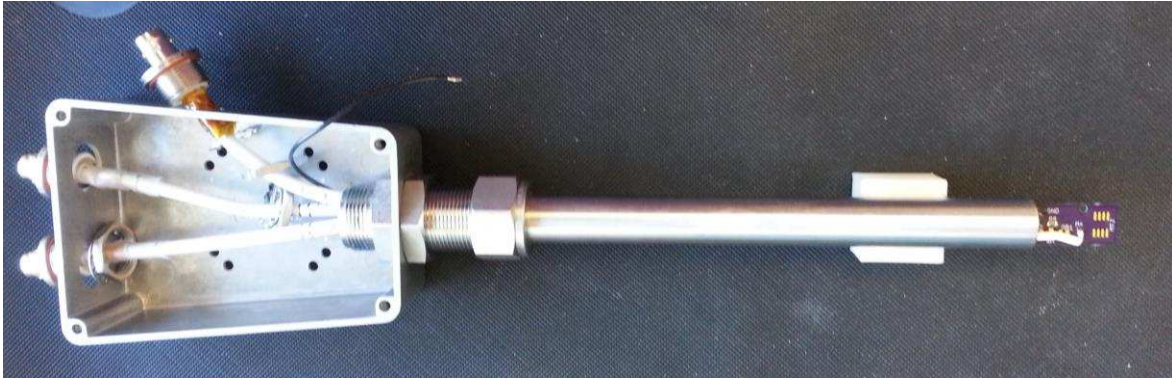
Figure 2.6: Two Axis Sensor Probe housing layout and design.
