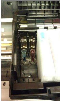
2. Fill pipette reservoirs with reagents
