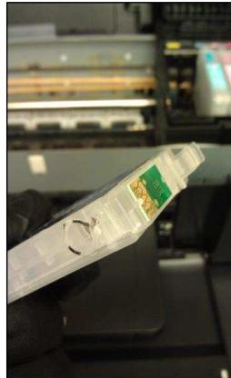
3. Drill holes in inkjet cartridge to fit over pipette reservoirs
