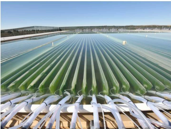
Figure 1. A) A closed algae system using plastic bags to protect culture from the outside environment. B) An open pond system exposed to the environment.
