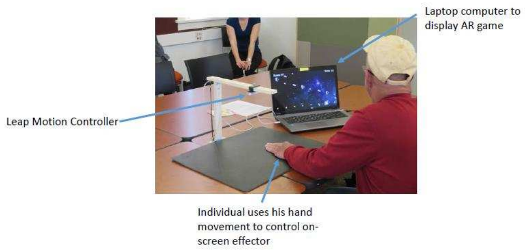
Figure S2: Components of the system
