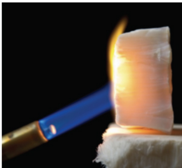
Figure 3.1. Alumina nanofiber block with the demonstration of fire retardancy 89
