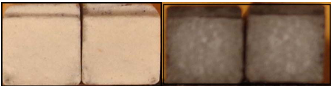
Figure 6.9. Fracture surface of CNF reinforced and treated at 650 °C in (a) oxygen and (b) nitrogen.
