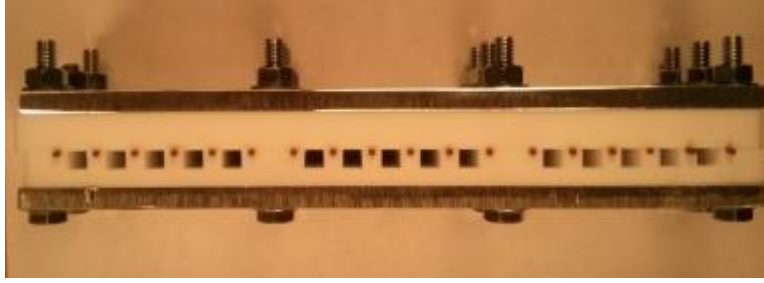
Figure 5.4. Assembly of a mold with rectangular slots for curing MEYEB in vertical orientation.
