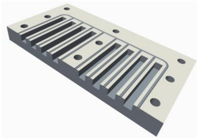
Figure 5.1. Molds for SEVNB specimens prepared using Acetal plastic
