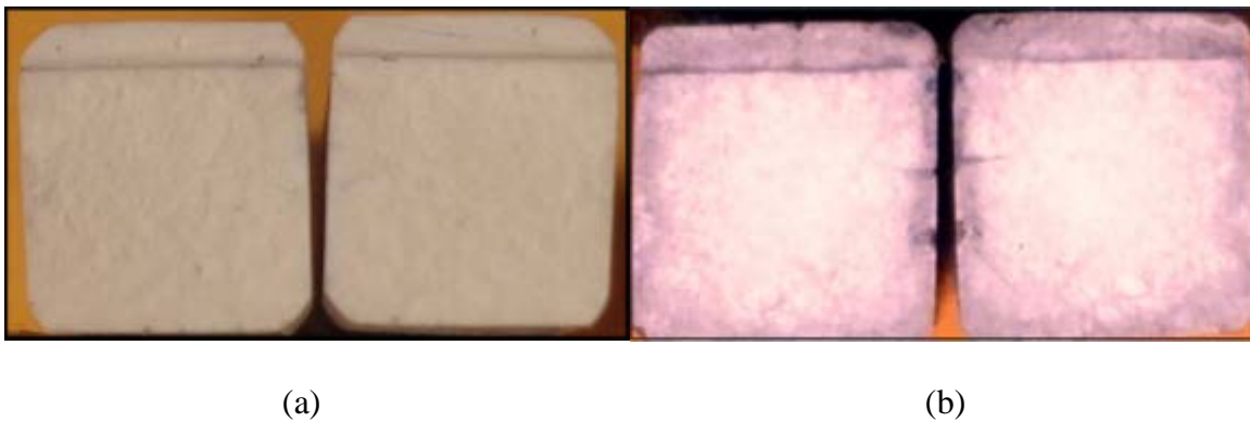
Figure 6.7. Fracture surfaces of ANF reinforced and treated at 760 °C in (a) oxygen and (b) nitrogen.
