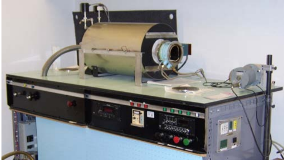
Figure 8.1. CVD furnace used to modify the sizing of the surface of fiber tow into a carbon deposited layer.
