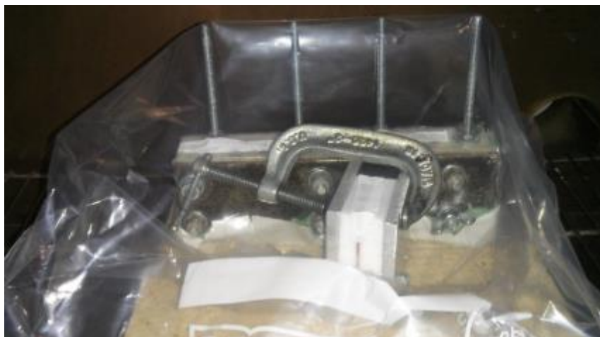
Figure 5.6 Assembly of the Mold with MEYEB in a sealed PE bagging.
