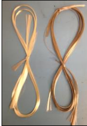
Figure 8.2. Nextel 610 fiber with (left) clean and (right) carbon deposited surface.
