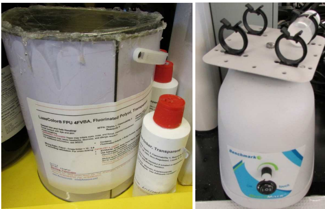
Figure 8.3: FPU components (left) and silica particles on vortex mixer (right).
