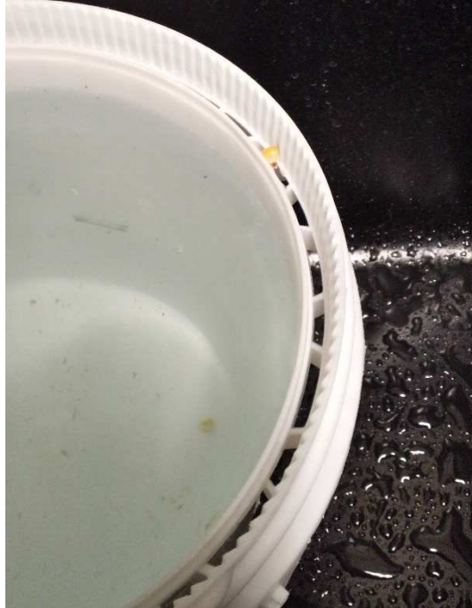
Figure 8.10: Corn washing bucket in sink with a trapped kernel.
