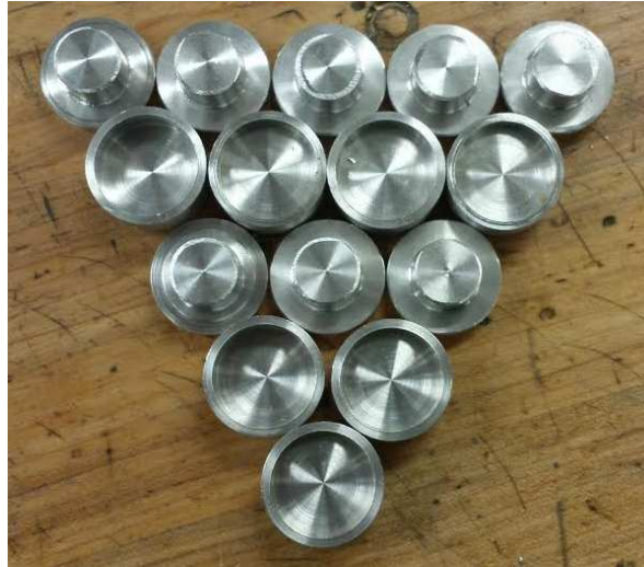
Figure 6.30: Fabricated disposable aluminum rheometer cups.
