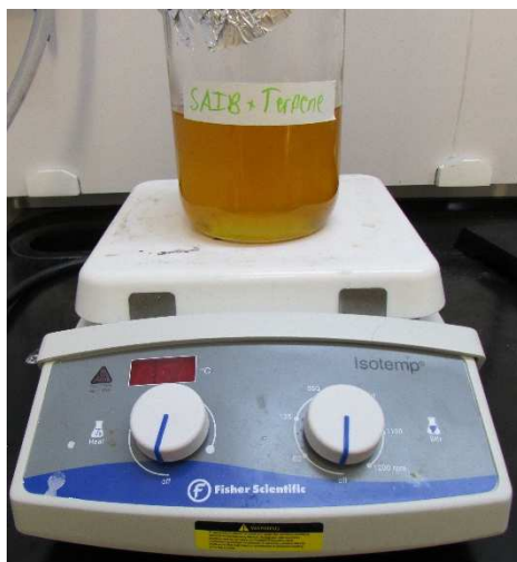
Figure 8.19: Syrup mixture on hot plate for mixing with magnetic stir bar.
