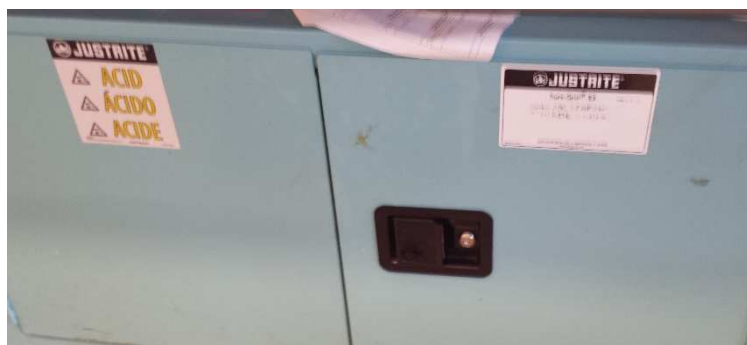
Figure 7.3: HF acid cabinet below fume hood.
