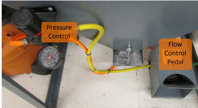
Figure 7.9: Pressure and flow control for bead blasting. Pull and rotate regulator dial to set pressure.
