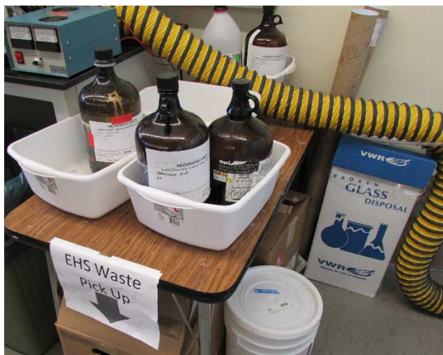
Figure 9.4: Haz-waste containment area with secondary containment and disposal boxes clearly marked.
