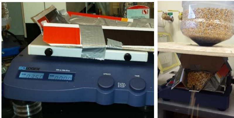
Figure 8.15: Shaker abrasion setup showing tilt and operation with hopper.
