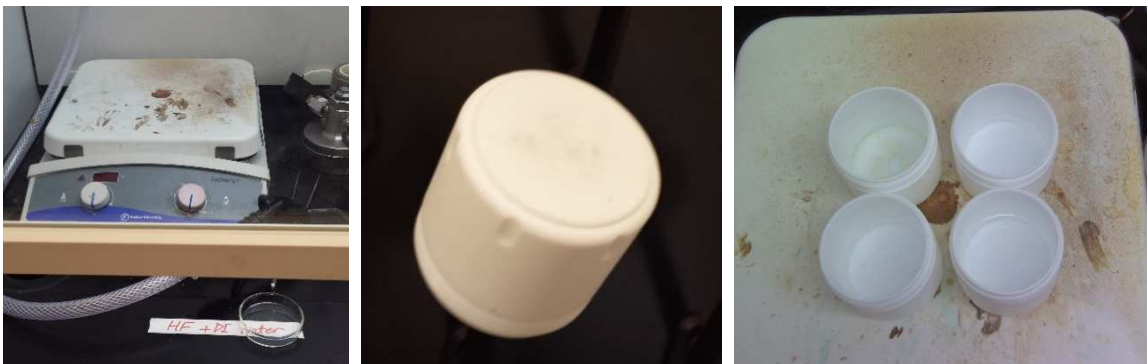
Figure 7.1: HF etching equipment with hot plate in fume hood and PTFE beakers on hot plate.
