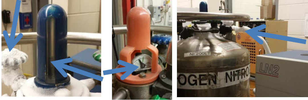
Figure 6.11: Liquid nitrogen valve, gauge, and connection.
