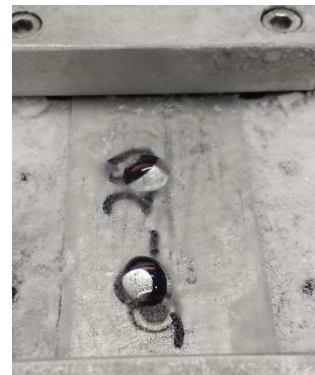
Figure 6.8: Anti-ice test on Peltier plate with DI drops.
