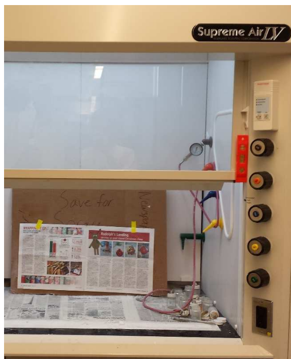
Figure 8.5: Spray coating fume hood with protective cardboard and newspaper.
