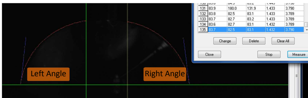
Figure 9.11: Contact angle lines shown on blackened screen showing droplet curvature.
