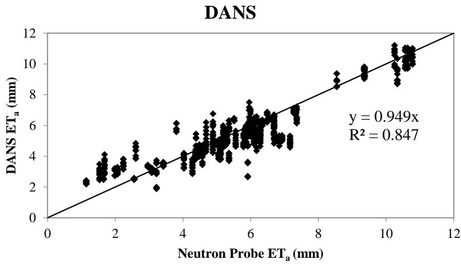
Figure 10. Scatterplot of DANS  $ET_a$  vs. Neutron Probe  $ET_a$  (mm),  $R^2 = 0.85$
