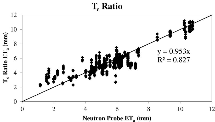
Figure 13. Scatterplot of T<sub>c</sub> Ratio ET<sub>a</sub> vs. Neutron Probe ET<sub>a</sub> (mm), R<sup>2</sup> = 0.83
