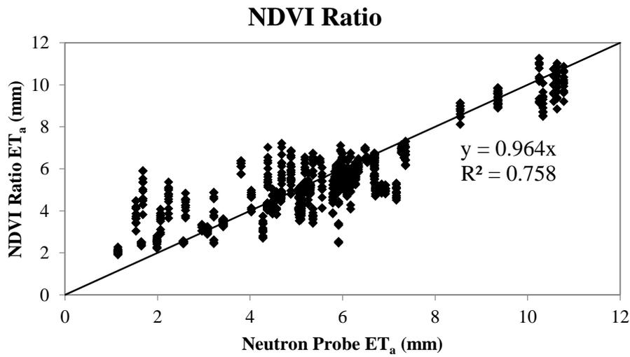
Figure 11. Scatterplot of NDVI Ratio  $ET_a$  vs. Neutron Probe  $ET_a$  (mm),  $R^2 = 0.76$
