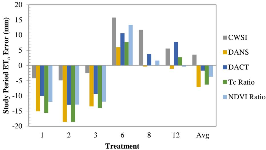
Figure 17. Error in study period  $ET_a$  (mm) of each  $K_s$  method for each treatment
