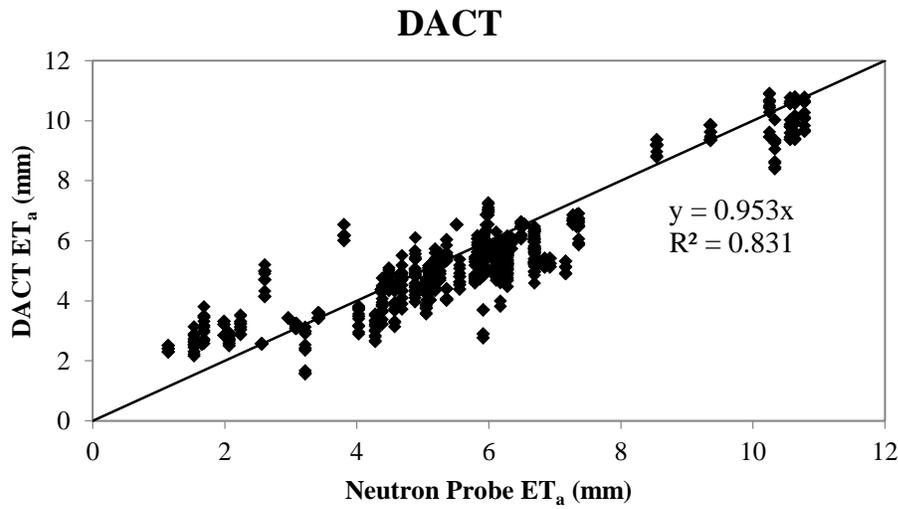
Figure 12. Scatterplot of DACT ET<sub>a</sub> vs. Neutron Probe ET<sub>a</sub> (mm), R<sup>2</sup> = 0.83
