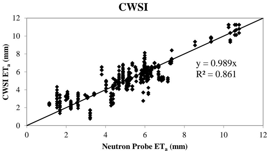
Figure 9. Scatterplot of CWSI  $ET_a$  vs. Neutron Probe  $ET_a$  (mm),  $R^2 = 0.86$
