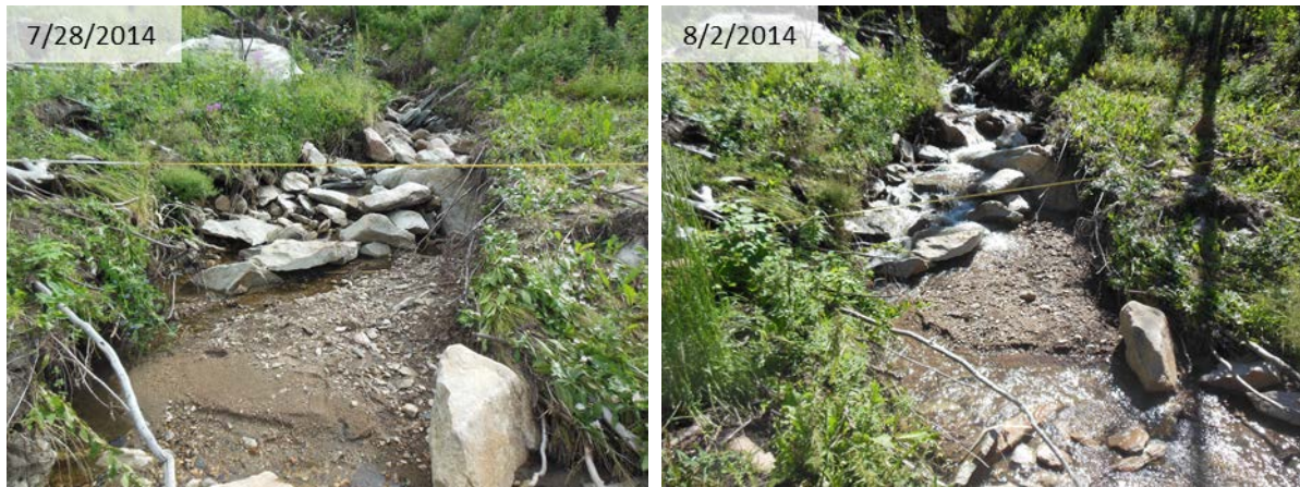
Figure 19: WPW XS 11p illustrating that bed material surveys reflect changes caused by the most recent event rather than trends through time.
