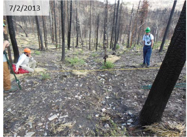
Figure 20: Examples of the mulch distribution and transport in WPW. Mulch distribution was variable and concentrated in topographic depressions such as swales and channels making it vulnerable to transport during the 7/1/2013 rain event.
