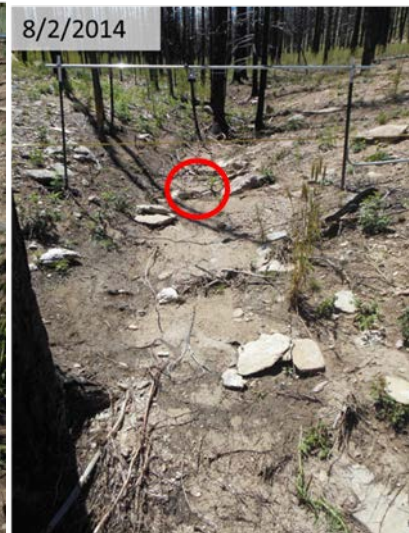
Figure 9: Repeat photographs of WPW XS 3e that illustrate the ephemeral channel is a temporary source and sink for sediment by alternating response between degradation and aggradation. Despite statistical insignificance, the direction of response appears to correspond to MI_{30} . The red circle in the photographs indicates a common bed location.
