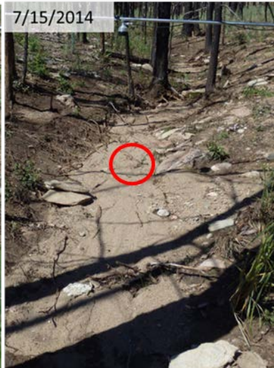
Figure 9: Repeat photographs of WPW XS 3e that illustrate the ephemeral channel is a temporary source and sink for sediment by alternating response between degradation and aggradation. Despite statistical insignificance, the direction of response appears to correspond to MI_{30} . The red circle in the photographs indicates a common bed location.
