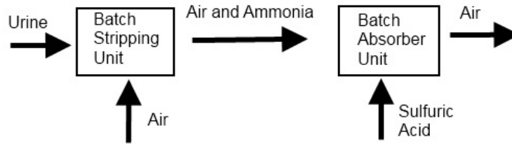
Figure 12 Simple process diagram for ammonia stripping
