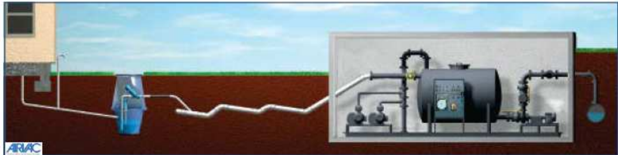
Pipes for vacuum sewers are installed in a saw-tooth or zigzag configuration to maintain a vacuum throughout the system.
