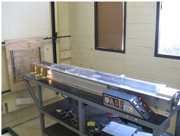
Figure 16 – Hail Impact Testing Configuration
