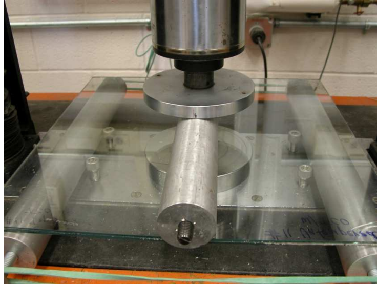
Figure 15 – Distributed Load Testing Configuration
