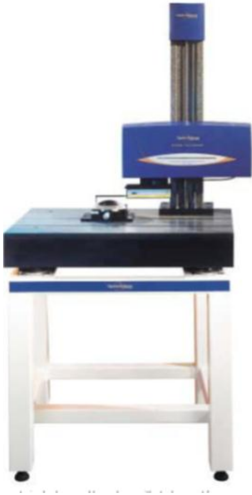
Figure 6: figure showing the measuring station of Taylor Hobson Profilometer
