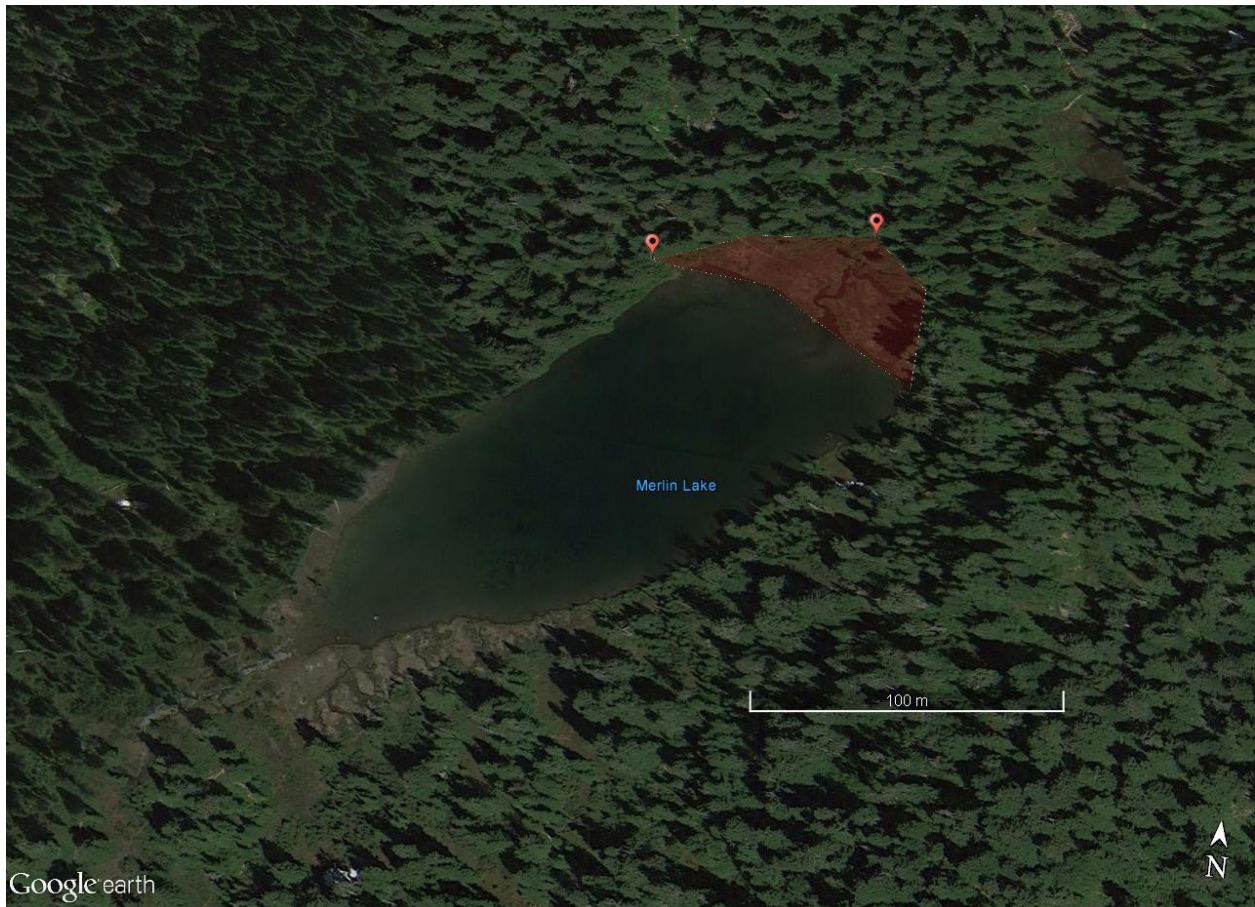
Figure 4: Google Earth image of the Merlin Lake Delta. Waypoints were placed along the margins of the delta that were difficult to identify using aerial imagery alone. The margins of the delta were traced in Google Earth to obtain a surface area for the delta (highlighted in red).
