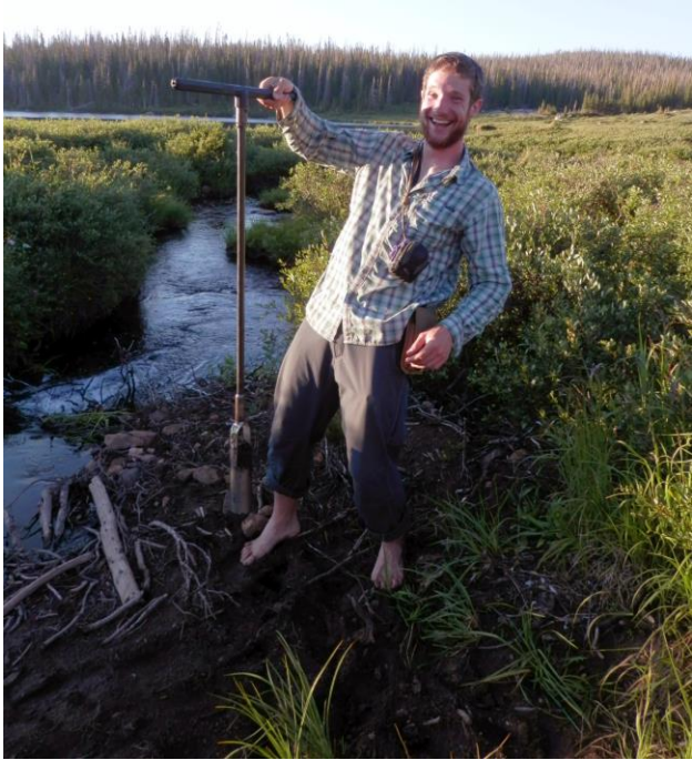
Figure 5: The author holding up an auger full of soil taken from a subalpine lake delta (A). The author coring a subalpine lake delta with an auger (B)
