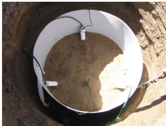
Figure A.12: Photograph of soil water samplers and sensors installed in lysimeters.
