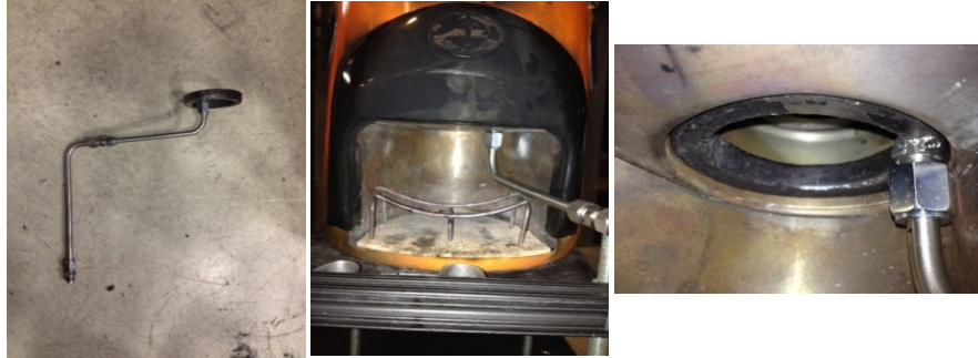
Figure 38. Chimney Ring Nozzle
