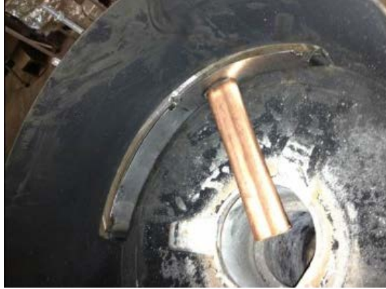
Figure 20. Conduit Routed from Stove Chimney to EGR Path
