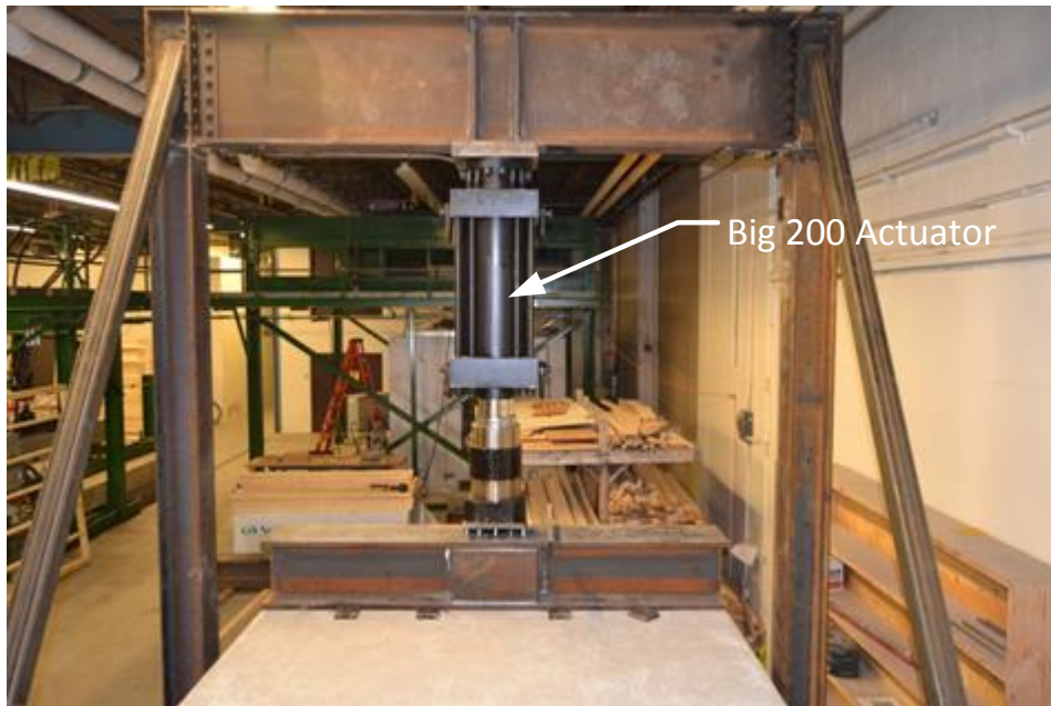
Figure 64 - 220 kip Actuator and Load Application Beam (May 2014)
