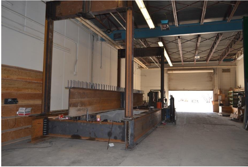
Figure 58 - Self-Reacting Load Frame – Upper Frames for Actuators (March 2014)
