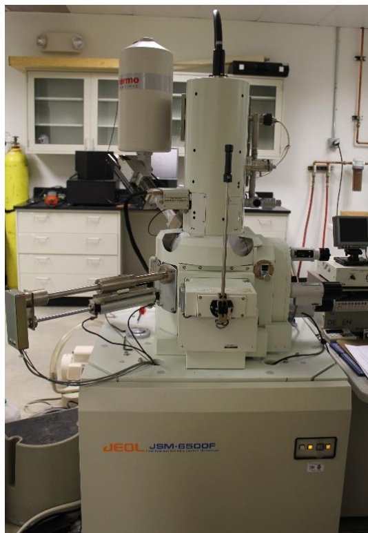
Figure 1.5: Scanning Electron Microscope with Energy Dispersive X-ray Spectroscopy Detector.
