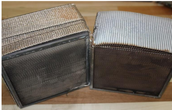
Figure 2.15: Catalyst modules. Emissions Module on Left and Material Sampling Module on Right (partially disassembled).
