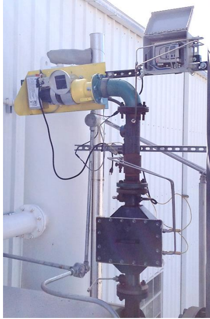
Figure 2.7: Final Catalyst Slipstream Assembly with Blower and Pitot Tube
