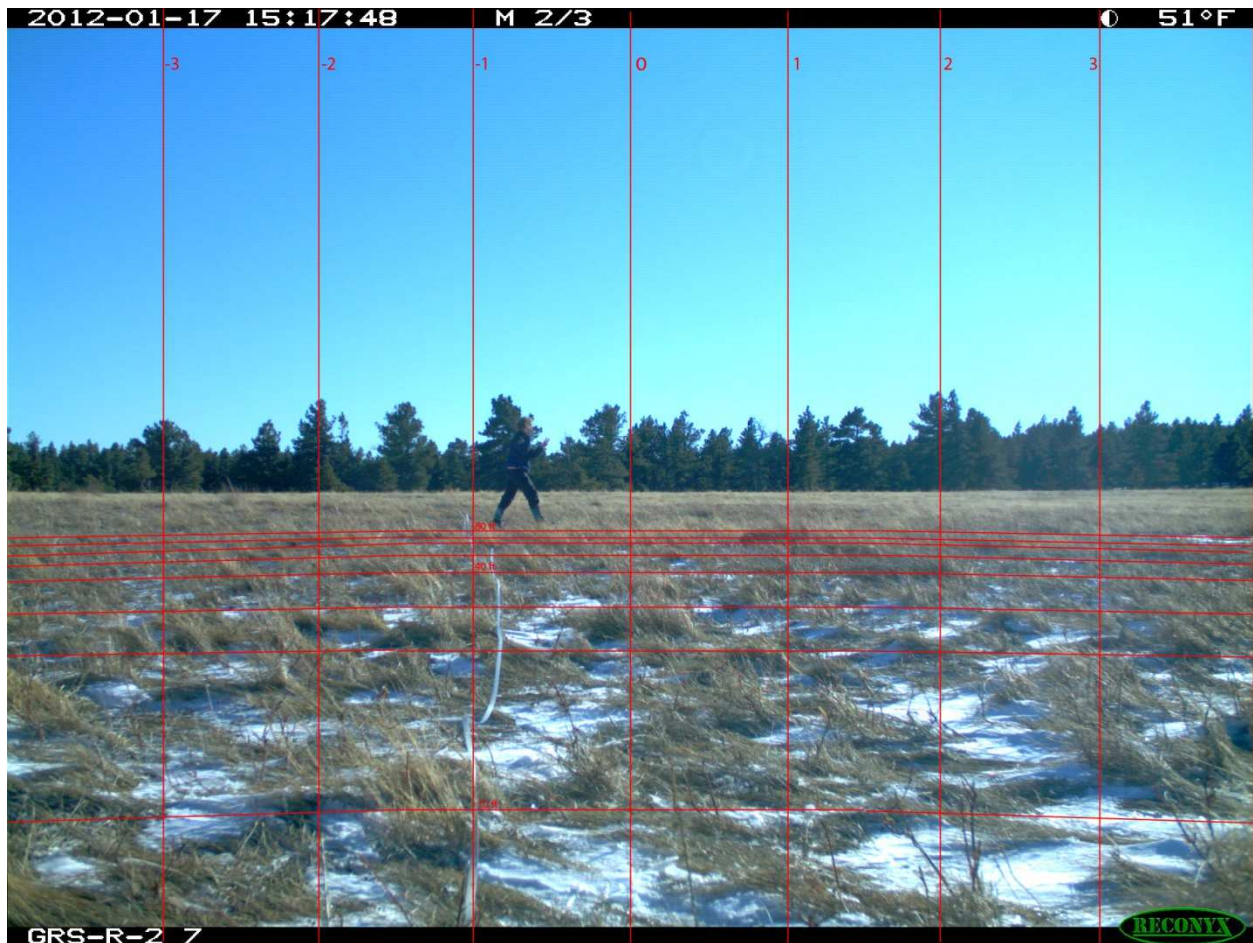
Figure A3.1. Compiled layer of horizontal and vertical measurement liens (red) overlaid on a photo of a technician making passes at the distance intervals. Horizontal lines indicate approximate distance intervals at 10 – 100 ft (3 – 30 m) in 10 ft (3 m) intervals. This particular example image has distance intervals marked at 10 ft intervals with a maximum distance of 80 ft. Vertical lines indicate the center or 0° (index 0), 5.04° (index 1), 10.08° (index 2), 15.11° (index 3), and 20.15° (photo edge) to the left (negative index) or right (positive index) of the center line.
