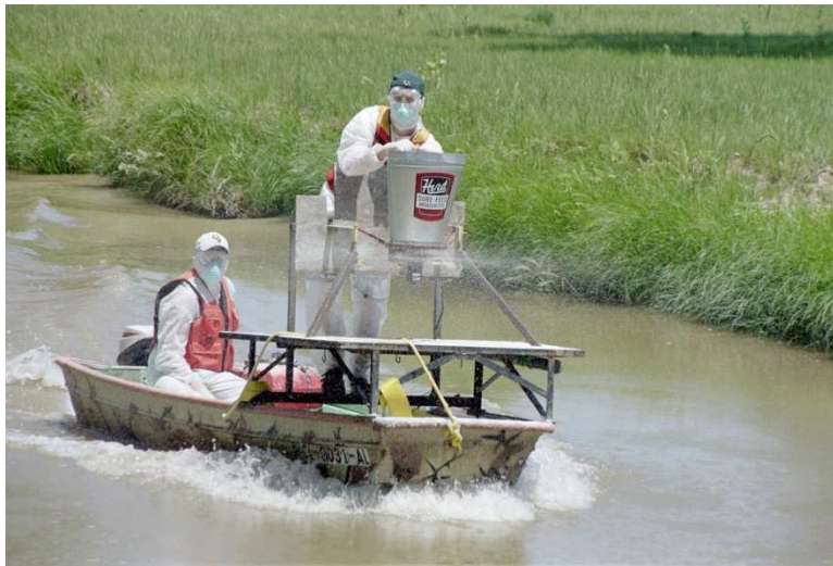
Figure 4-1 PAM application with a boat on the RFH Canal using an automatic spreader
