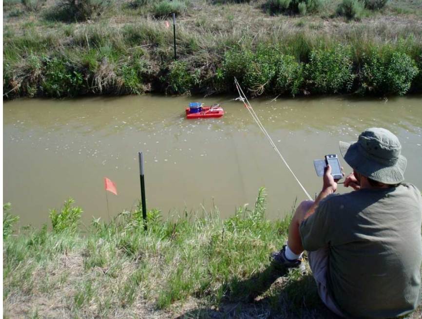
Figure 3-6 ADCP StreamPro measurement on the Lamar Canal (2006) looking toward the right bank
