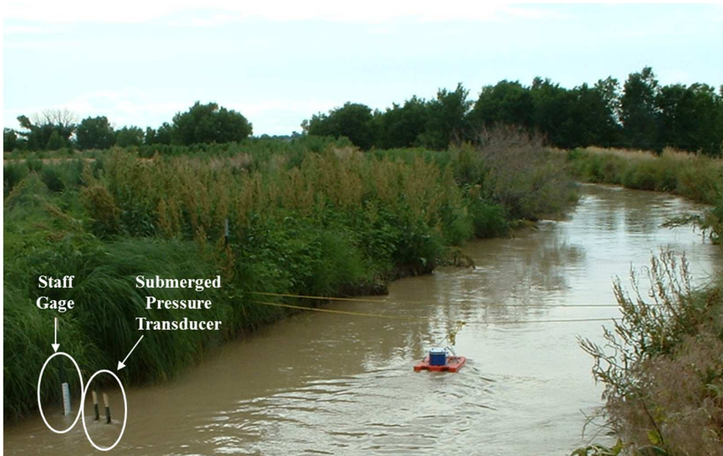
Figure 3-13 Picture of a staff gage and location of a submerged pressure transducer at Site 202
