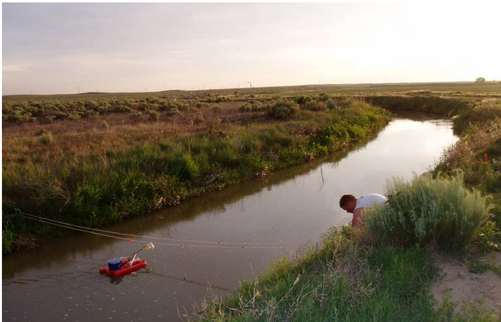
Figure 3-7 ADCP StreamPro measurement on the Lamar Canal (2006) looking upstream
