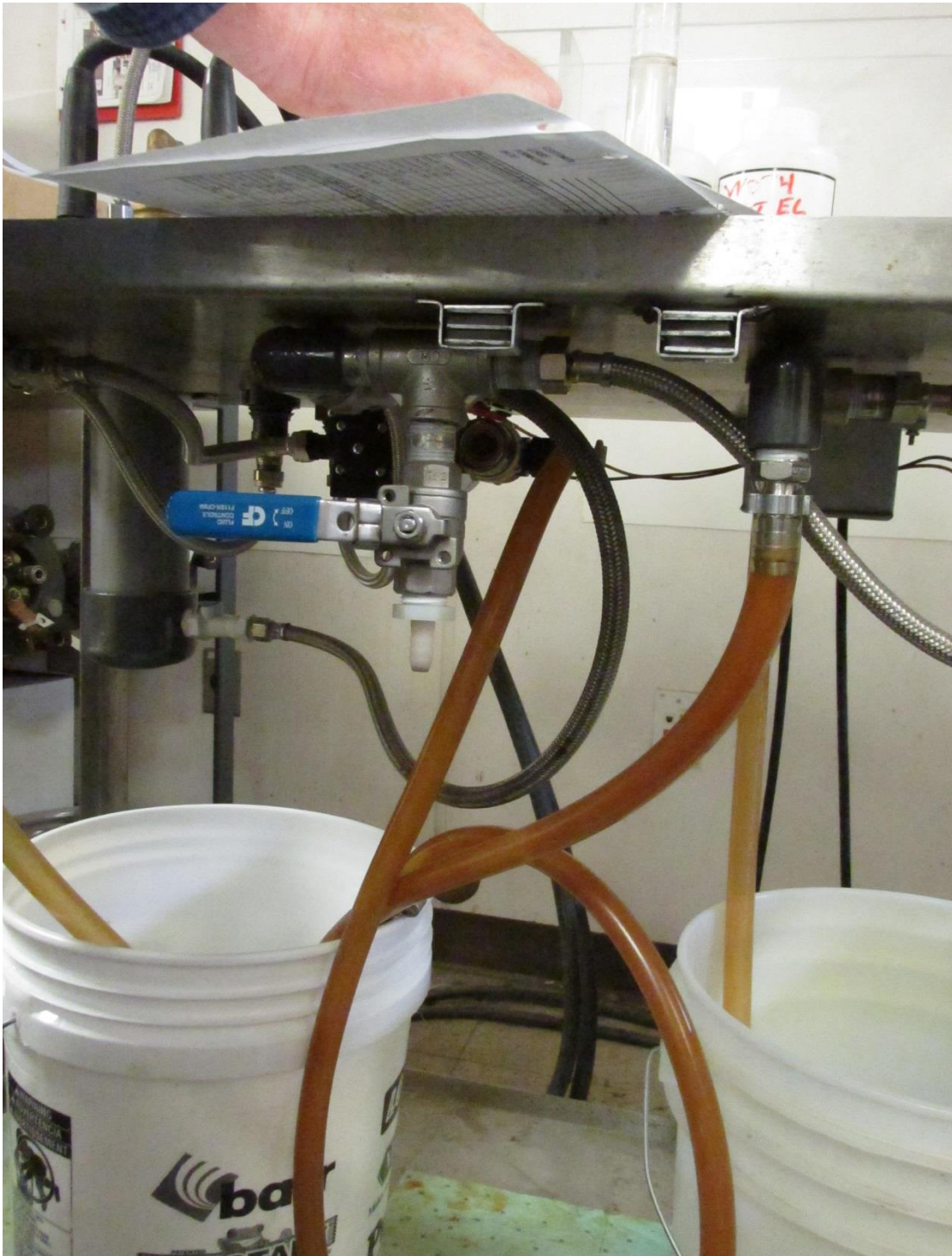
Figure 32. Underside view of EC bench unit. Effluent of EC cell on left, raw water sample in the white bucket on the left, treated water sample flows to the right bucket.
