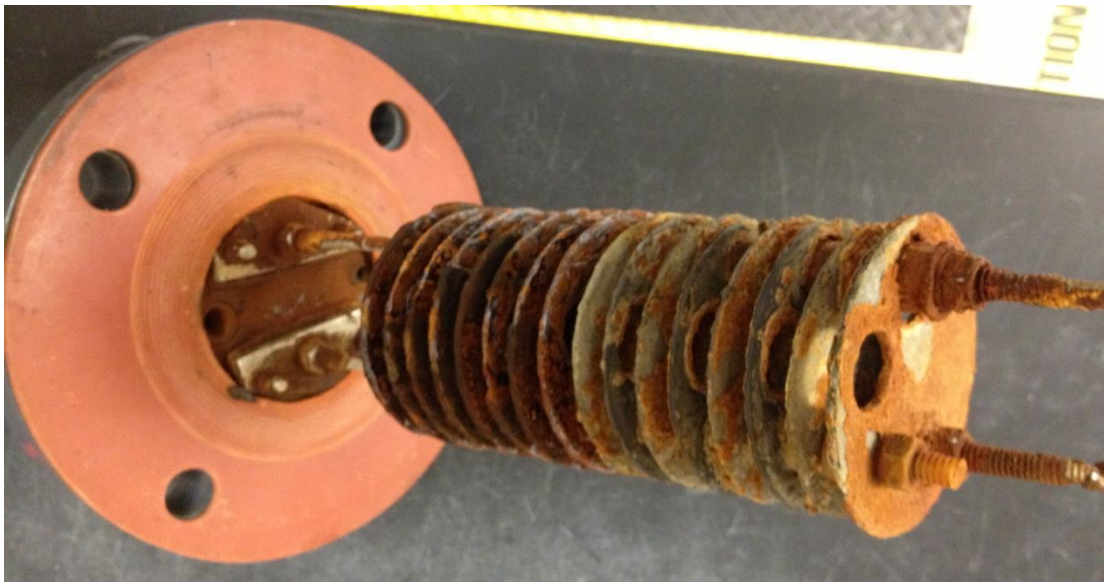
Figure 18. Example of the EC cell and plates before use. In this case, all plates are aluminum. However, in the experiment, a combination of aluminum and iron plates were used.
