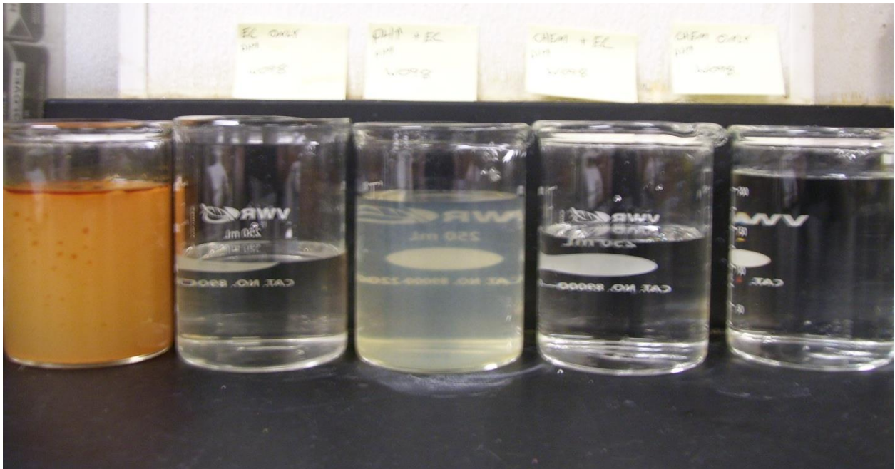
Figure 22. Day 90 raw and post treatment samples. The raw sample is on the far left with EC directly to the right. The CC sample is on the far right. The two samples in the middle were not used for analysis in the Thesis.
