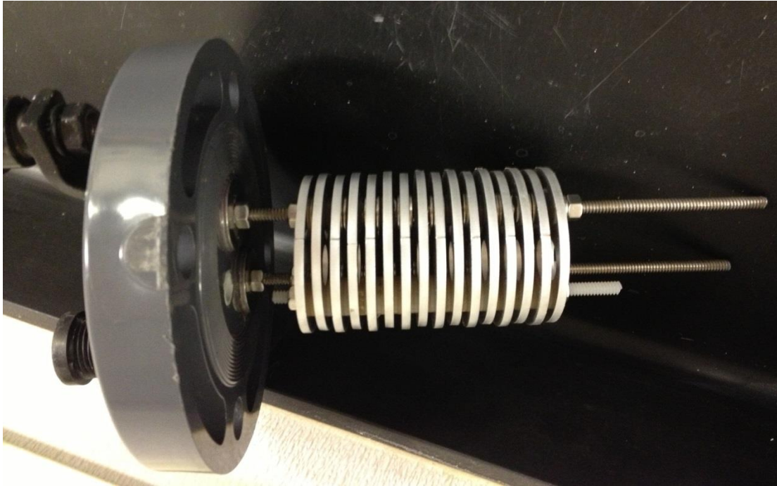
Figure 18. Example of the EC cell and plates before use. In this case, all plates are aluminum. However, in the experiment, a combination of aluminum and iron plates were used.
