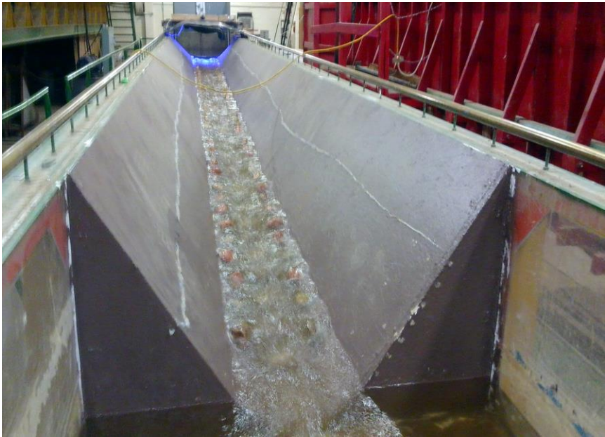
Figure 4-1. —The model rock ramp constructed at the Colorado State Engineering Research Center (left photo) and an example of a low-flow notch in a fishway in a small Colorado stream (right photo). The low-flow notch in the fishway is 21.3 m long and has a slope of 4.5%. The model rock ramp fishway was constructed in a 1.2-m wide flume, and average water depths were 0.11 m.
