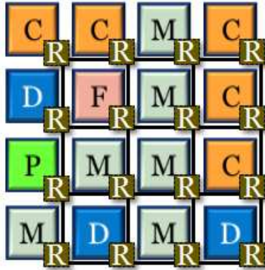
Figure 4 Networks-On-Chip (NoC), C: processor core, M: memory banks D: digital signal processors F: floating point processors P: global power management module
