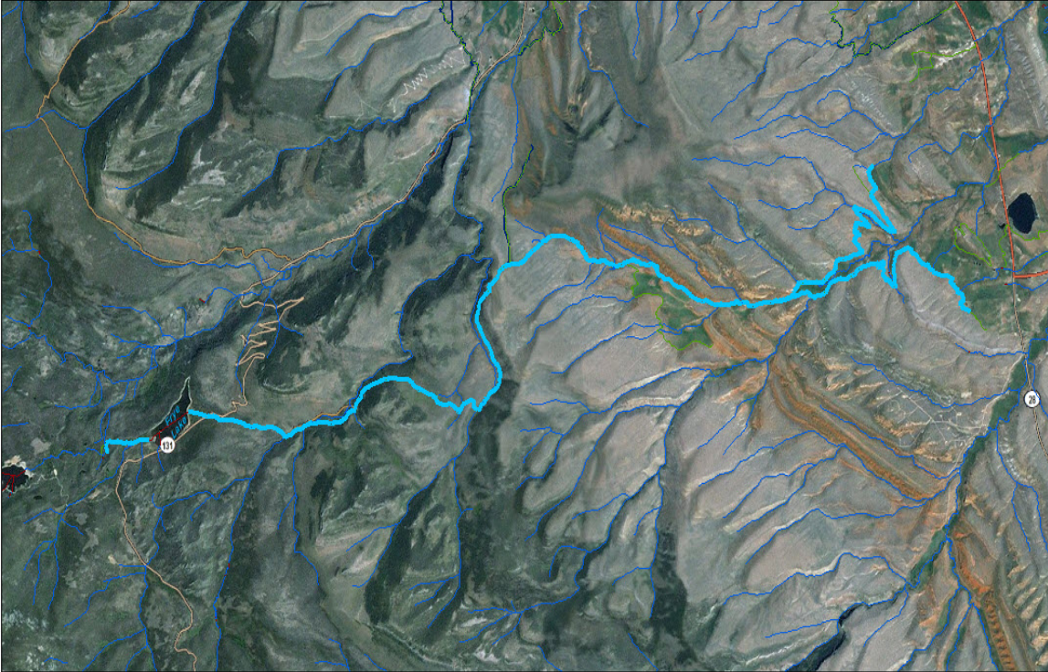
Figure 1. Enterprise Ditch near Lander, WY. Heavy blue line shows the alignment of a small ditch which intercepts drainage from a 14-square mile basin.
