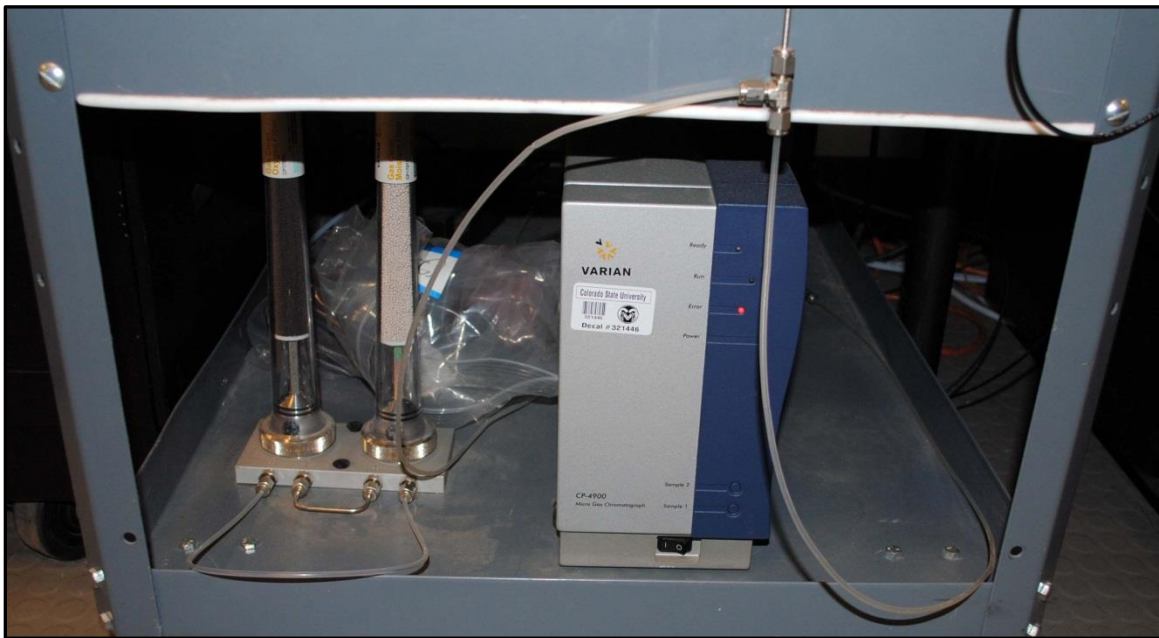
Figure 24. Varian CP – 4900 gas chromatograph for measuring fuel gas composition.
