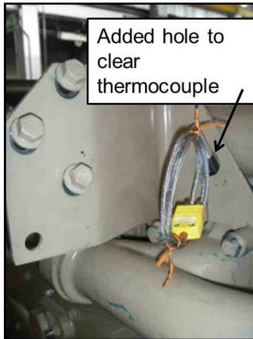
Figure 19. Modified Turbocharger Support Bracket.
