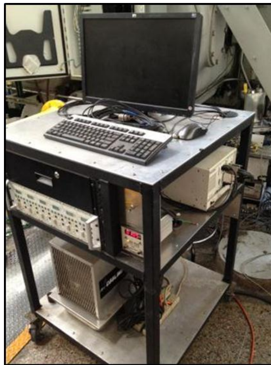
Figure 25. CSU Combustion Analyzer Cart.
