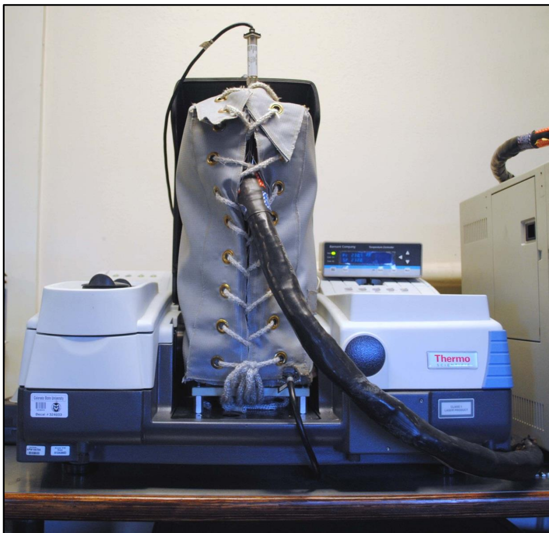
Figure 23. Nicolet 6700 Fourier Transform Infra Red spectrometer for measuring HAPS and other constituents.
