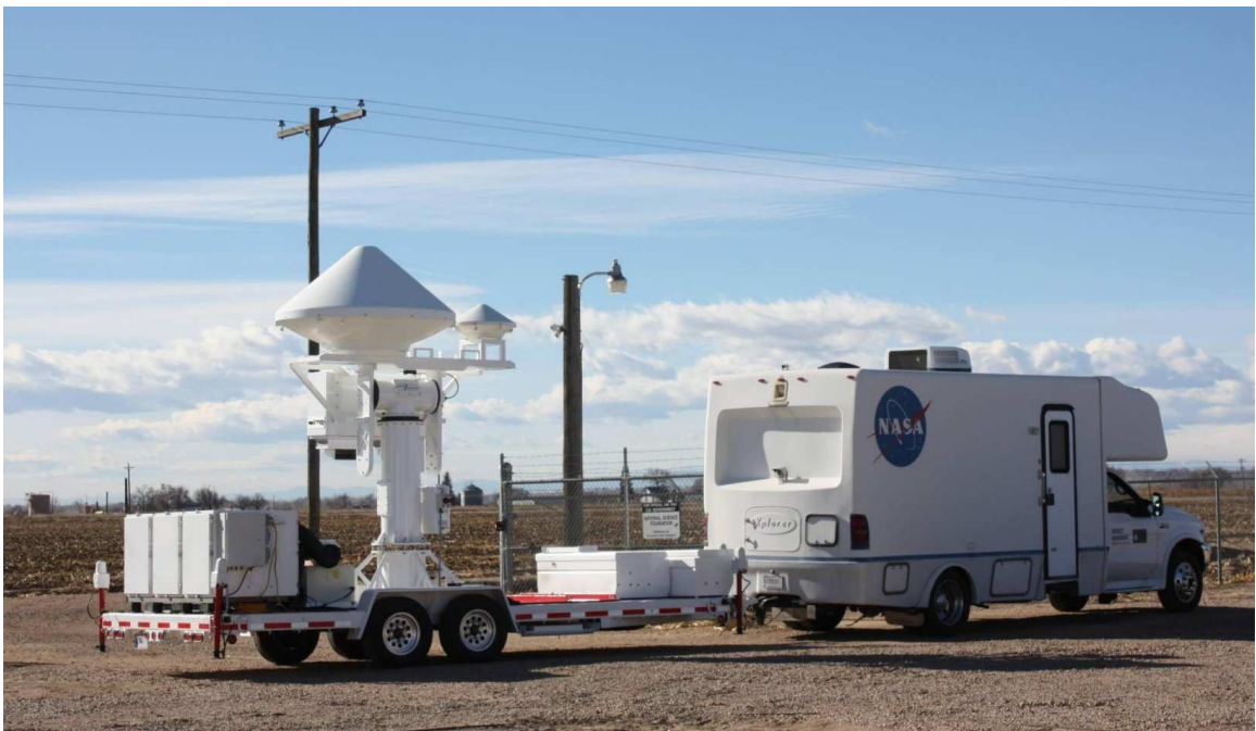
Figure 6.3: The D3R pedestal is mounted on a trailer that can be towed by a van-sized vehicle. This photograph was taken on Dec 09, 2010 during the antenna assembly phase at CSU-CHILL site.
