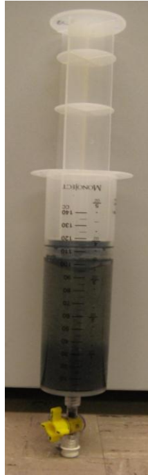
Figure 3.1 Batch reactor for determining hydrolysis kinetic rates
