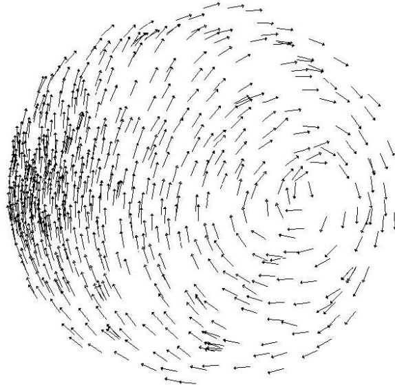
Figure 3.29 Velocity vectors for vertical open surface tank system operating at 0.000946 \text{ m}^3/\text{s} (15 gpm) about a xy -plane 1.5 m from the bottom surface.
