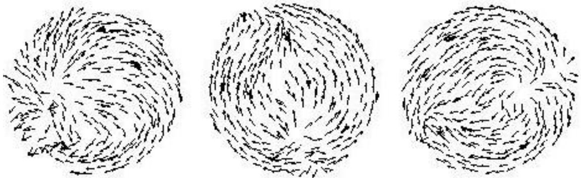
Figure 3.13 Velocity vectors for the 3 series tank system operating at 0.001262 m 3 /s (20 gpm).
