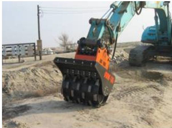
Figure 6. 36" vibratory roller (MBW, Inc.) attached to the end of an excavator arm.
