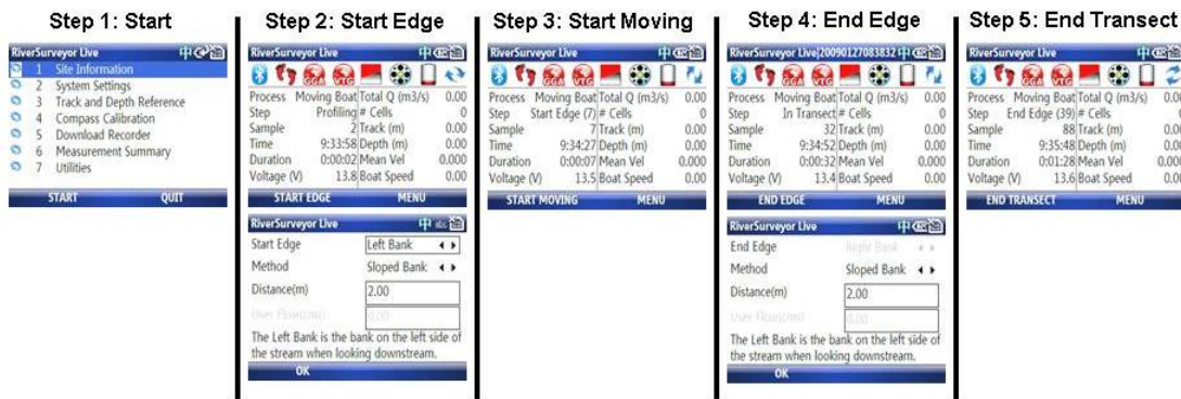
Figure 5. Five steps in completing a discharge measurement
