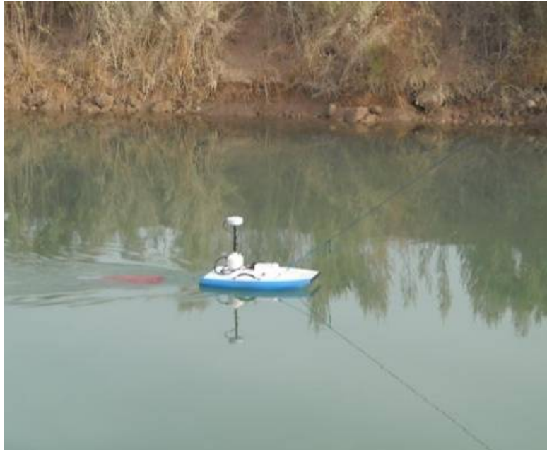
Figure 4. SonTek RiverSurveyor assembled on SonTek Hydroboard
