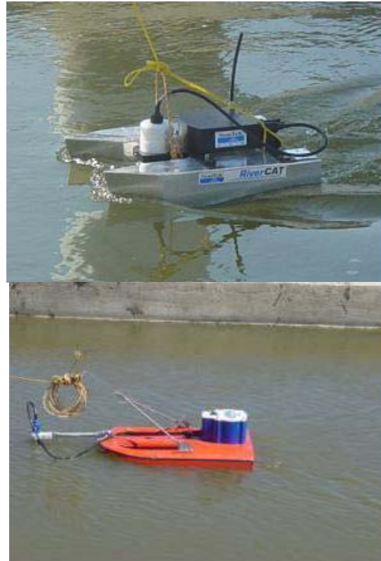
Figure 1. Boat-mounted Acoustic Doppler Profilers collecting flow rate and cross-sectional measurements in irrigation canals
