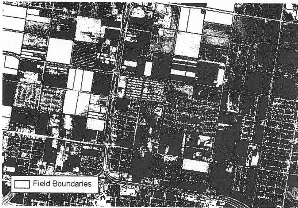
Figure 2. Water account boundaries created in GIS using an aerial photograph as a guide. This photograph is from a USGS DOQQ (digital ortho quarter quad), a high resolution photograph that has been registered.
