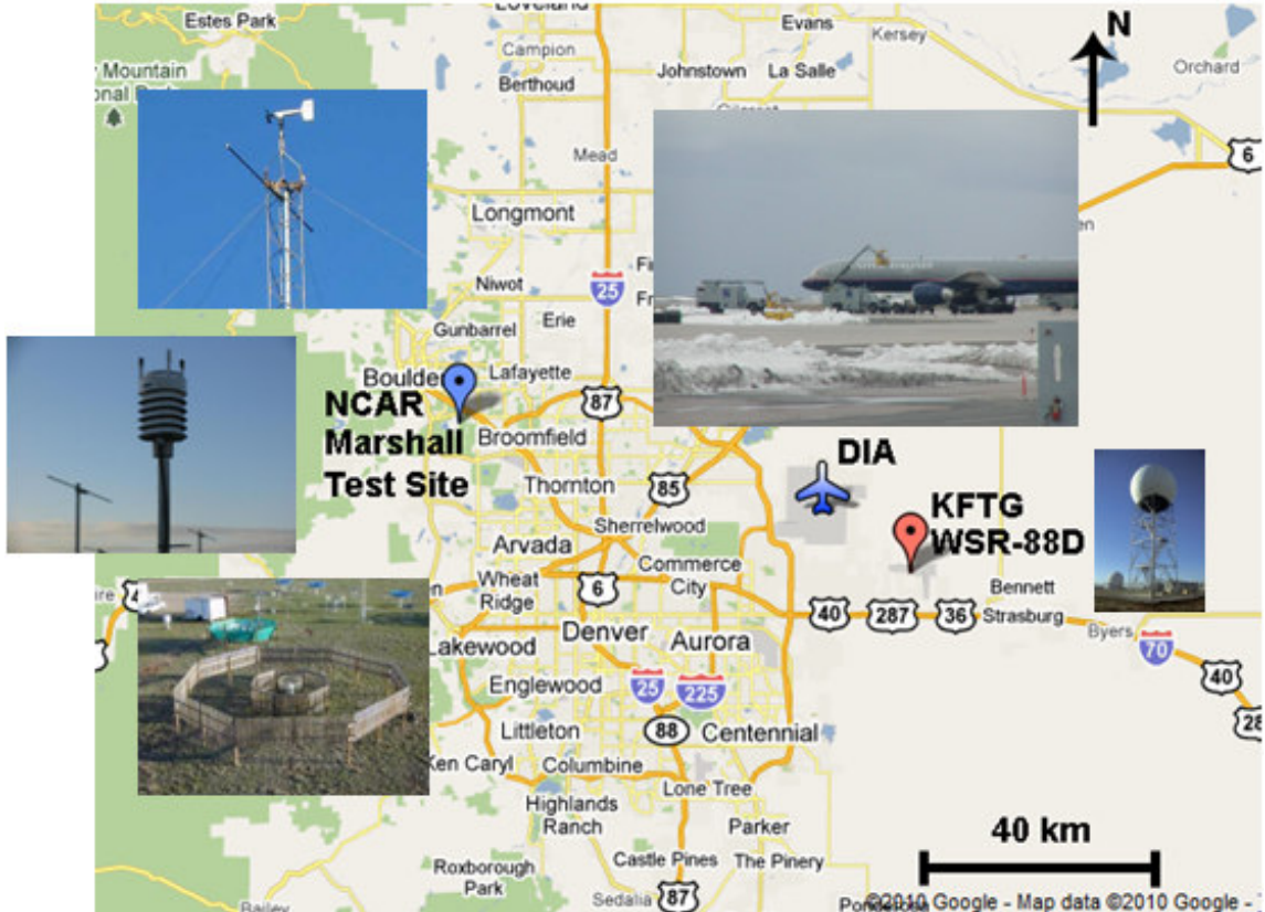
Figure 34. Map of the WSDDM evaluation sensor layout.
