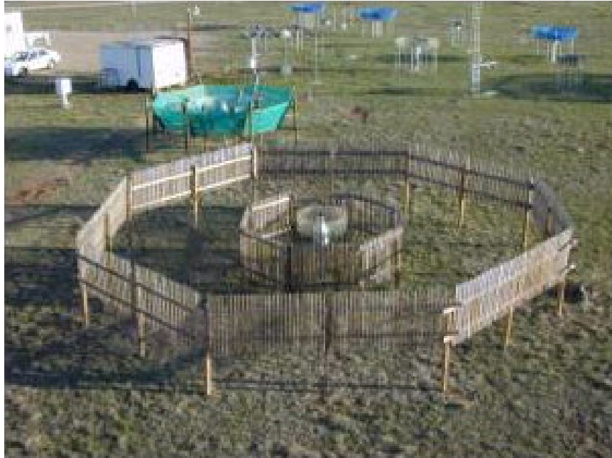
Figure 33. The WMO DFIR Geonor gauge located at the NCAR Marshall Test Site.
