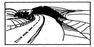
Often, the most difficult part of roadway design is to visualize three-dimensionally from the traditional horizontal plan and vertical profile method. Horizontal and vertical discontinuity can result in any or several of the following conditions, broken-back vertical curve, roller-coaster effect, short sag on long horizontal curve, or a vertical curve at the beginning of a horizontal curve. There are issues of Horizontal/Vertical Integration which are too complicated to address in this article.
