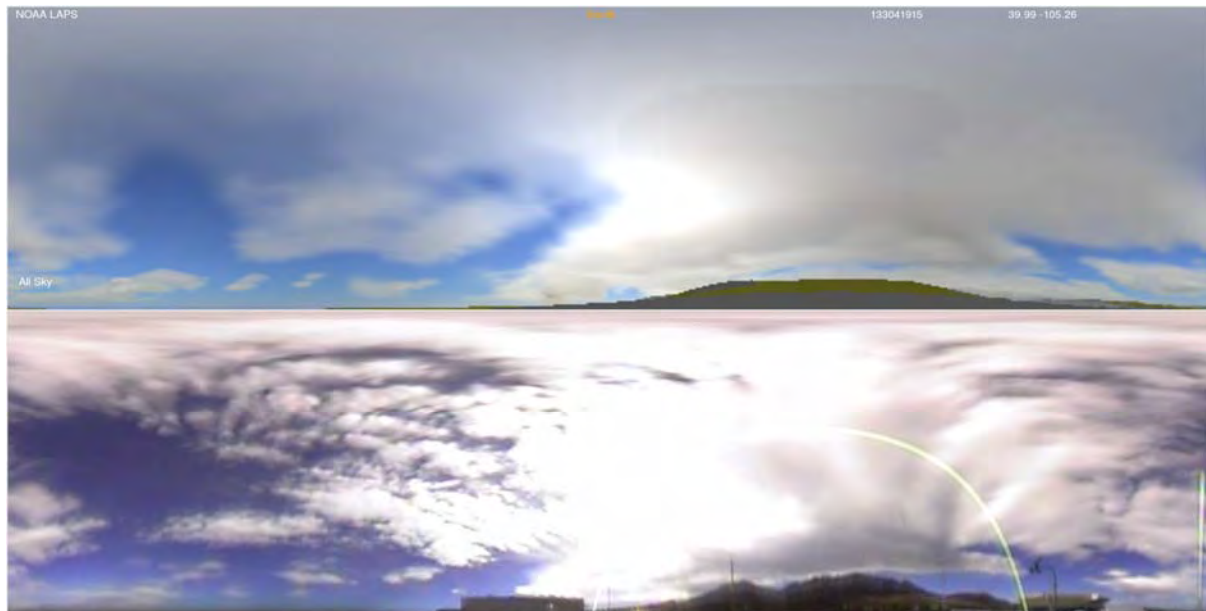
Figure 2. Simulated All-Sky image generated from 1km LAPS analysis data (top) compared with all-sky image from the DSRC rooftop camera (bottom).
