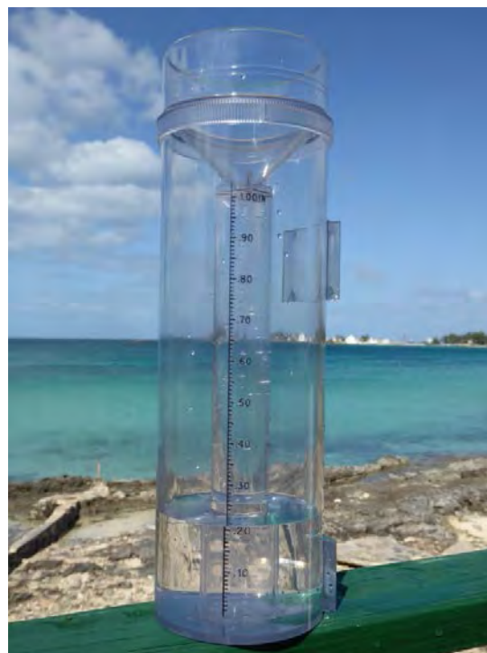
Figure 2. CoCoRaHS 10.2cm (4") gauge
