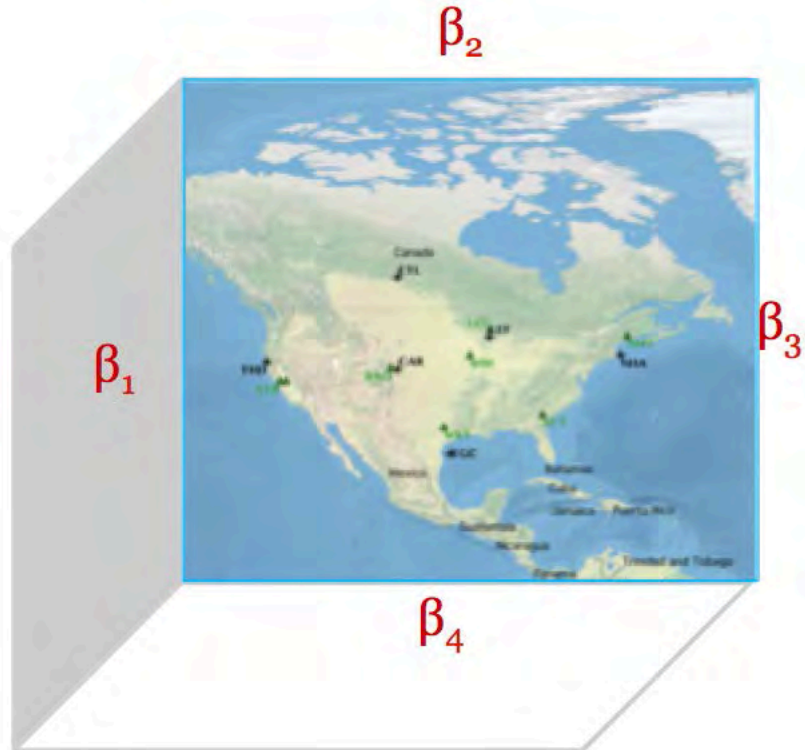
Figure 1. The schematics of the boundary condition optimization scheme: the four parameters \beta_1 , \beta_2 , \beta_3 , \beta_4 represent the mean bias corrections for the four sides of our domain within consecutive 10-day windows.
