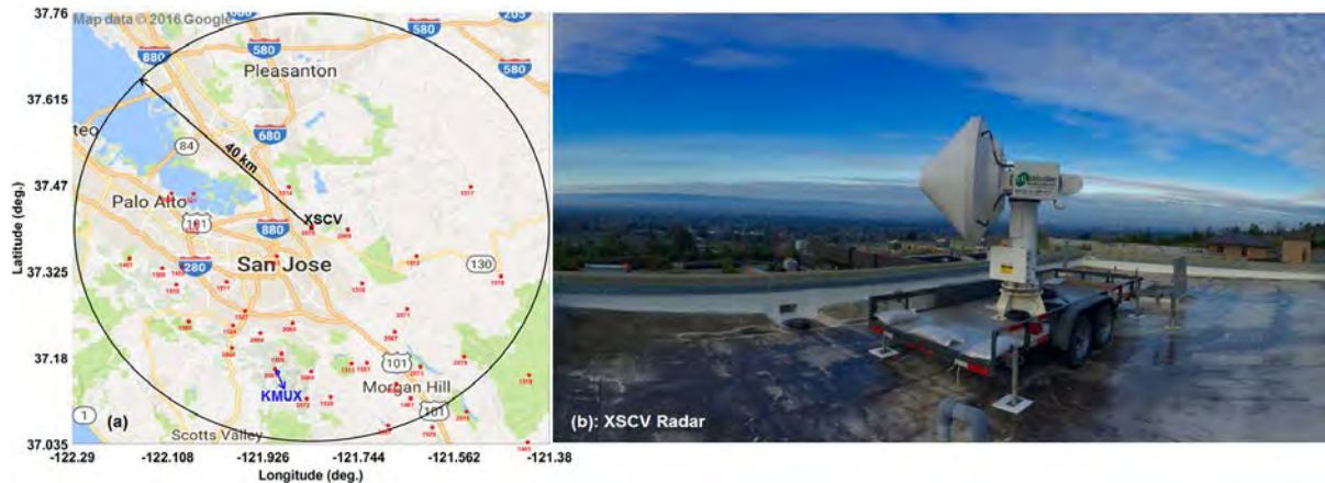
Figure 1. (a) Location and coverage map of X-band dual-polarization XSCV radar in Santa Clara, CA; (b) a photo of the XSCV radar during the deployment. The coverage range is 40km. The red dots in (a) denote the locations of rainfall gauges operated by SCVWD. The blue square in (a) illustrates the location of S-band KMUX NEXRAD radar. (for Project 1)
