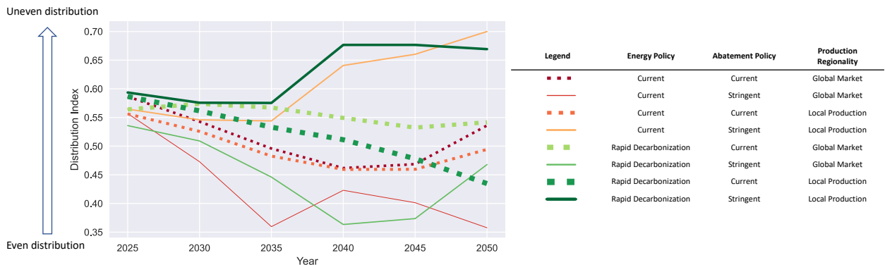
Figure 4.4. Trends in distribution index for regional distributions of emissions relative to demand, for all cases. Dashed lines show Current Abatement Legislation cases. Line widths and dash widths are linearly proportional to 2025-2050 total emissions from mining and smelting. The distribution index shows how regionally emissions are distributed compared to where demand occurs. A value closer to zero indicates emissions are collocated with demand. Values closer to one indicate most emissions are comparatively concentrated in fewer regions compared to demand. ‘Current’ under Energy Policy and Abatement Policy refers to ‘Current Energy Policies’ and ‘Current Abatement Legislation’, respectively.
