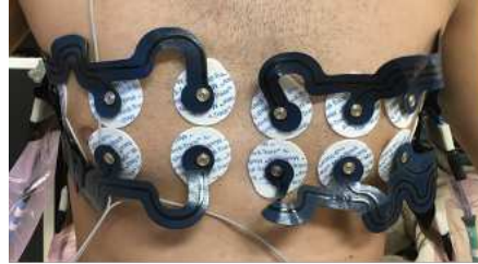
Figure 7.1: A photo of 32 electrodes arranged in two rows of 16 on the WEAT (wearable electrode applicator textile) belt designed by GE Research. This photo is taken from [55]. The EIT system used on this healthy volunteer is the GE GENESIS EIT system [52].
