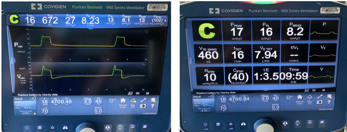
Figure 1.2: Two screenshot of the Puritan Bennett 980 Series Ventilator. Both screenshots come from one patient and are discussed in chapter 9. The screenshot on the left includes curves like pressure and airflow rate. The screenshot on the right includes the resistance value, compliance, and minimum and maximum pressures.
