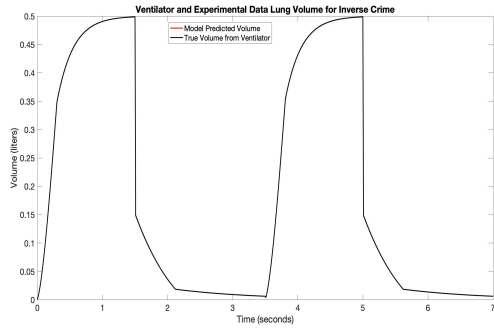
Figure 5.2: Left: Comparison of the synthetic volume curve (black) and from the inverse problem (red). The 2–norm relative error is 8.8e - 7\% . Right: Reconstructed resistance vector curve of [5.67, 6.79, 7.17, 6.79, 5.9, 4.6, 3, 1.47, 0.05] (red) and true resistance vector (blue).
