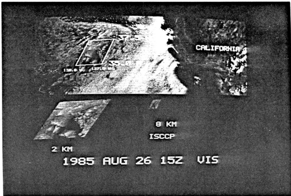
Figure 9: Cloud patterns observed in GOES visible imagery at full resolution (2 km per pixel) and sampled for the ISCCP continuing data archive (8 km).
