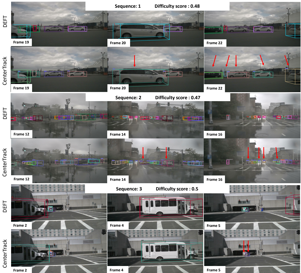
Figure 4.4: Qualitative results comparison between DEFT and CenterTrack [7] on nuScenes. Each pair of rows shows the results comparison for one sequence. The color of the boxes represents the identity of the tracks. Red arrows point at tracking errors (identity switches). Notice that DEFT is more robust to occlusions and large inter-frame displacements.
