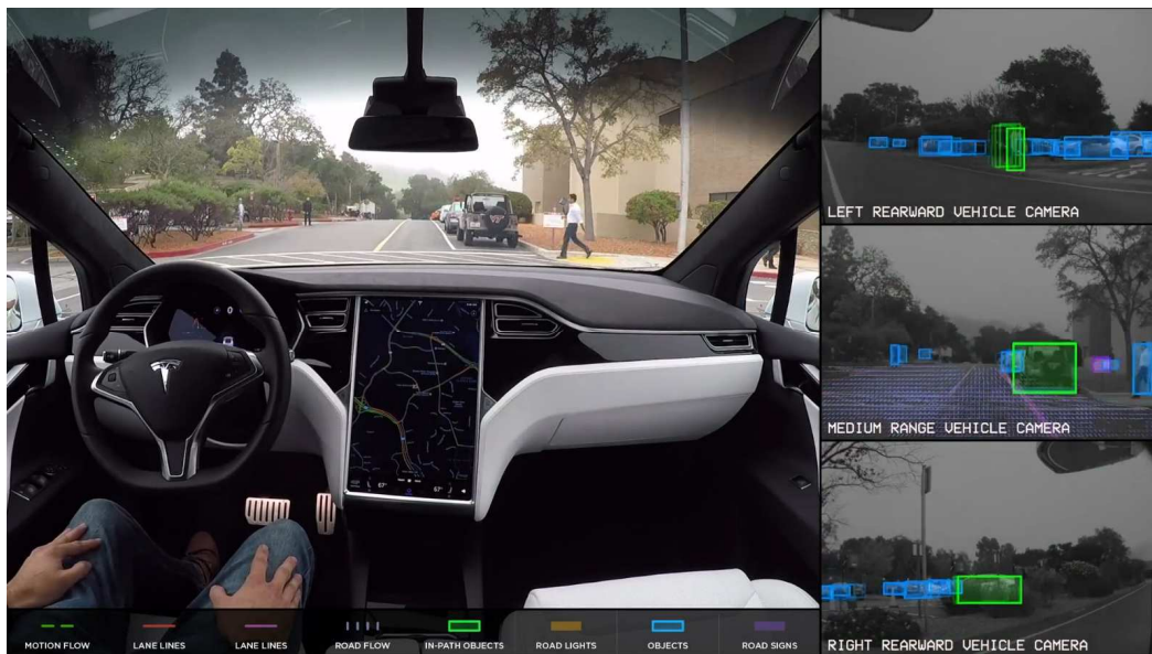
Figure 5 The Tesla's autopilot perceived view of surroundings using different cameras [9].
