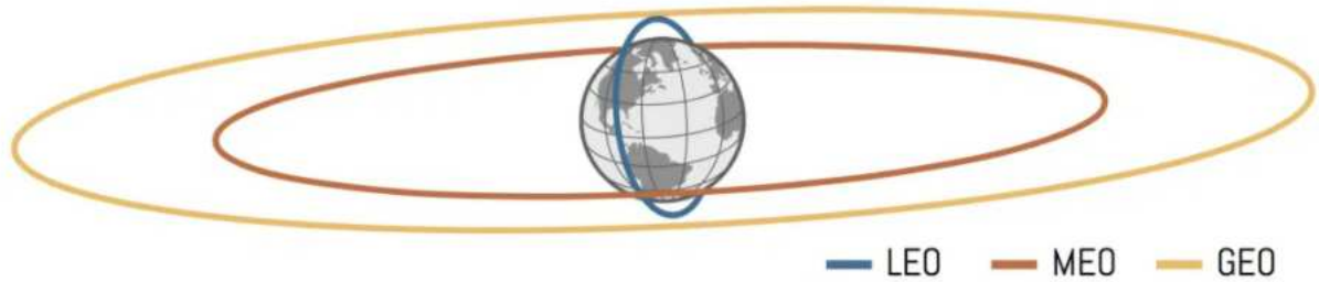
Figure 2.1: Popular Orbit Regimes. Low Earth Orbit (LEO) is shown in blue, Medium Earth Orbit (MEO) is in red, and Geosynchronous Orbit (GEO) is in yellow [2].
