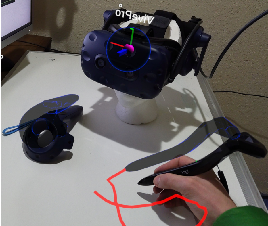
Figure A.4: Poorly synchronized Vive-Pro client and controllers as viewed through the HoloLens 2. Legend: The faint blue / gray controller outlines are the rendered controller representations to visualize cross-device synchronization, the red is the line drawn using the VR-Pen.
