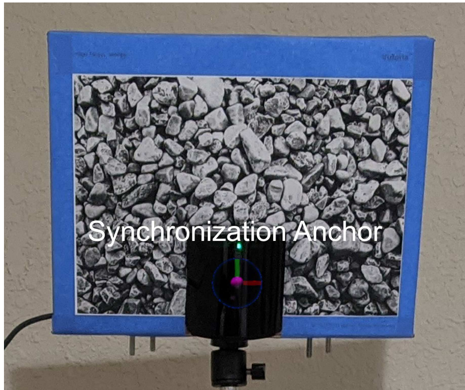
Figure A.1: Vuforia image target mounted on top of Vive-Pro Base Station 2.0, synchronization anchor position adjusted down from the center of the image target to the base station center.
