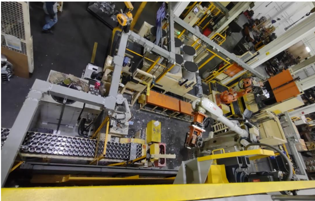
Figure 28: Example extraction cell with multiple robots and post-die cast processing (photo permission from Mercury Marine)
