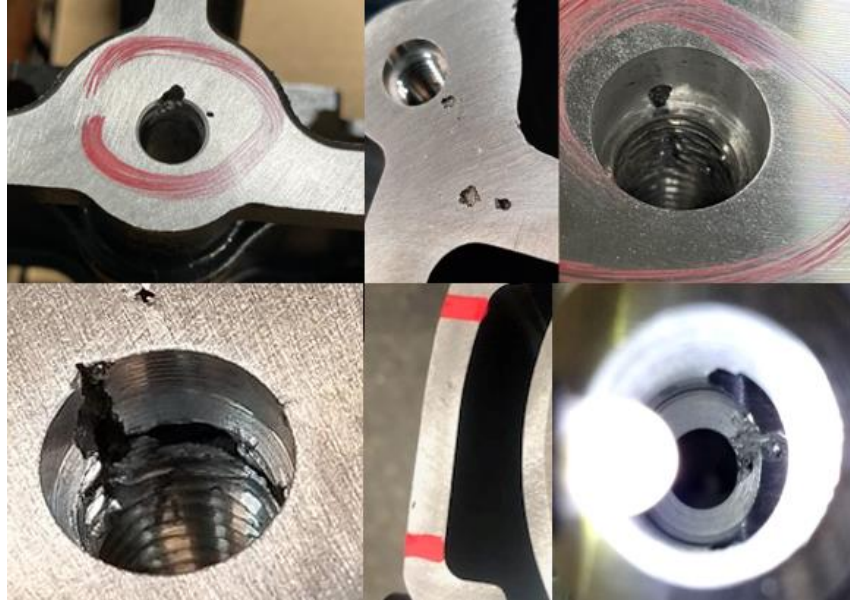
Figure 36: Examples of HPDC porosity
