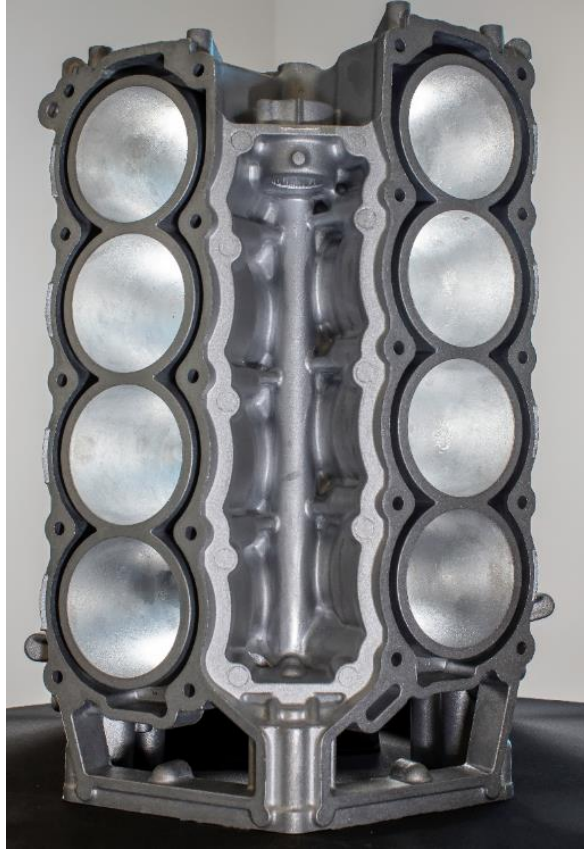
Figure 2: Example V8 engine block die casting (photo permission from Mercury Marine)
