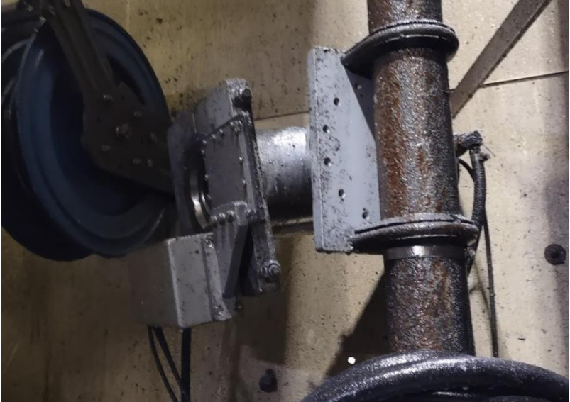
Figure 26: Thermal imaging camera in production die cast environment (photo permission from Mercury Marine)
