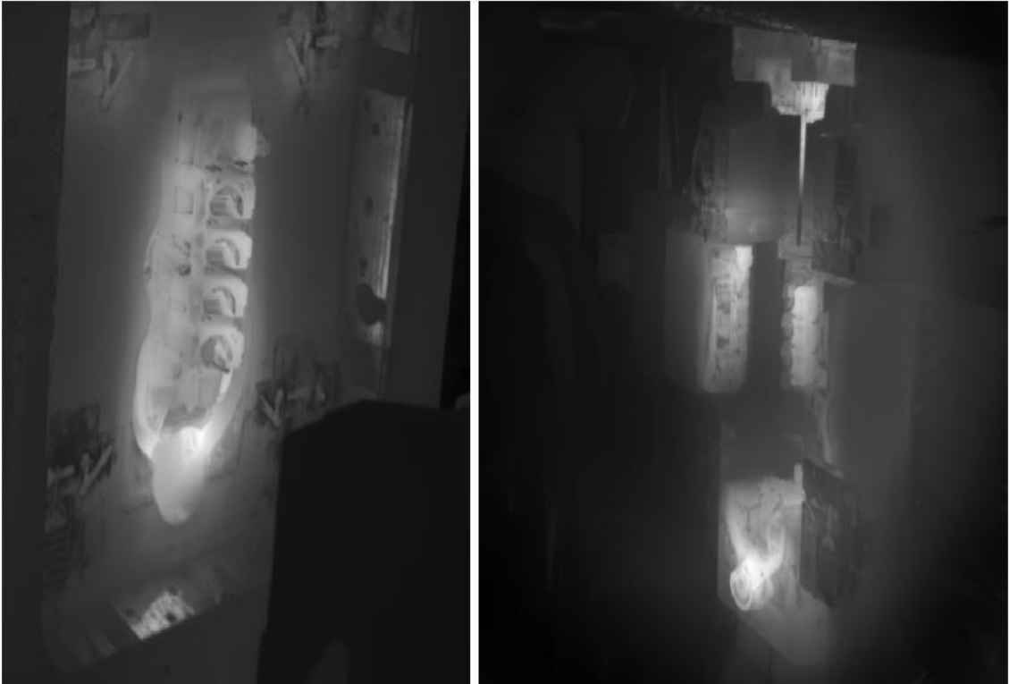
Figure 27: Example thermal image on stationary half (left) and moving half (right) (photo permission from Mercury Marine)
