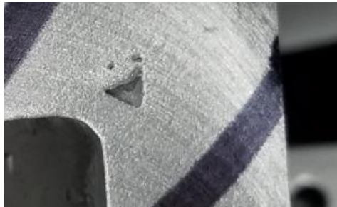
Figure 60: Gate break-in defect
