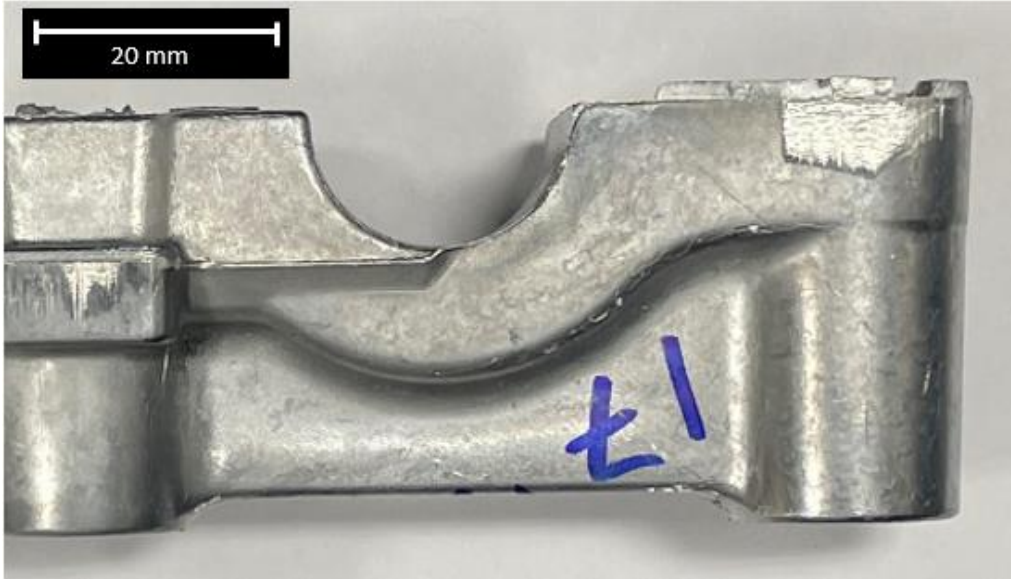
Figure 29: Sawed sample casting for X-ray
