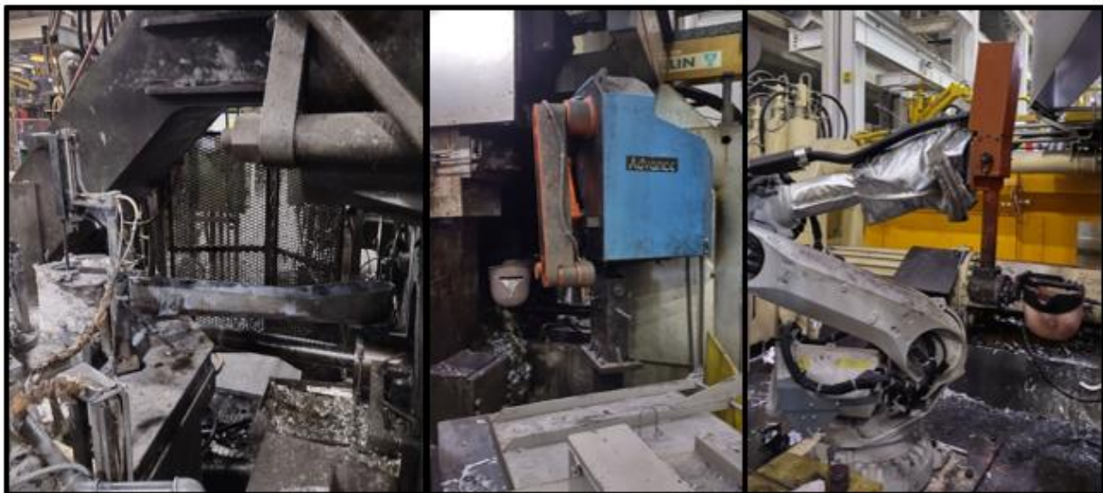
Figure 3: Metal delivery: dosing furnace (left), 2-axis ladle (center), and 7-axis robot ladle (right) (photo permission from Mercury Marine)
