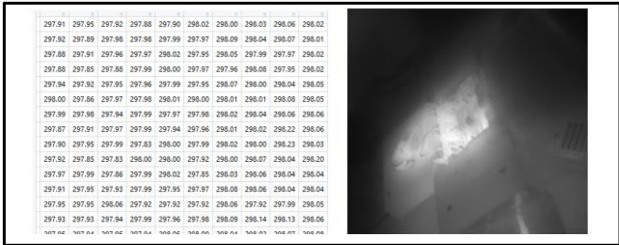
Figure 80: Thermal image temperature matrix and grayscale image
