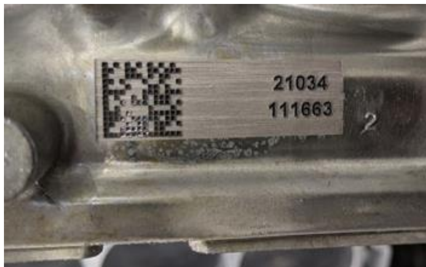
Figure 55: Example 2D laser barcode on a die casting (photo permission from Mercury Marine)
